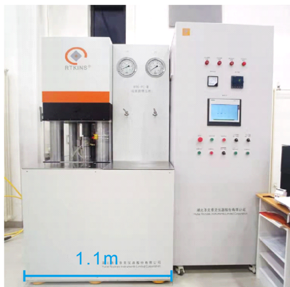
FIG. 5. Piston-cylinder press at HPSTAR.
