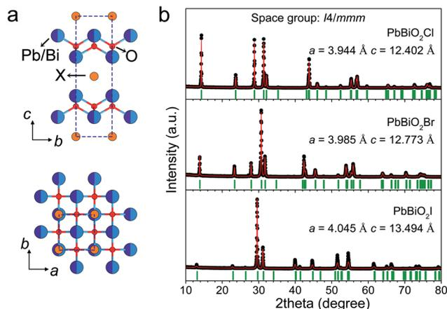
Fig. 1 Crystal structures of  $\text{PbBiO}_2\text{X}$  ( $\text{X} = \text{Cl}, \text{Br}, \text{I}$ ). (a) The tetragonal structure viewed along  $[100]$  and  $[001]$ . (b) Rietveld refinement results of the  $\text{PbBiO}_2\text{X}$  samples with space group  $I4/mmm$ . In (b), experimental: black circle; simulation: red lines; Bragg reflections: olive bars.
