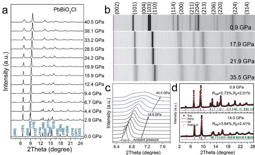
Fig. 3 Selected angle-dispersive XRD patterns of  $\text{PbBiO}_2\text{Cl}$  with incident  $\lambda = 0.4340 \text{ \AA}$  at RT (a). (b) 2D images of  $\text{PbBiO}_2\text{Cl}$  at 0.9 GPa, 17.9 GPa, 21.9 GPa and 35.5 GPa, respectively. (c) The evolution of (101) reflections under pressure. (d) Two refinement results for  $\text{PbBiO}_2\text{Cl}$  at 0.9 GPa and 14 GPa.
