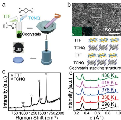
**Fig. 1** (a) The schematic diagram for the fabrication of the TTF–TCNQ bulk samples. (b) The SEM image of the TTF–TCNQ pellet and the stacking structure of the TTF–TCNQ cococrystals. (c) The Raman spectrum of the TTF–TCNQ crystals. (d) The XRD data of the TTF–TCNQ crystal under different temperatures.
