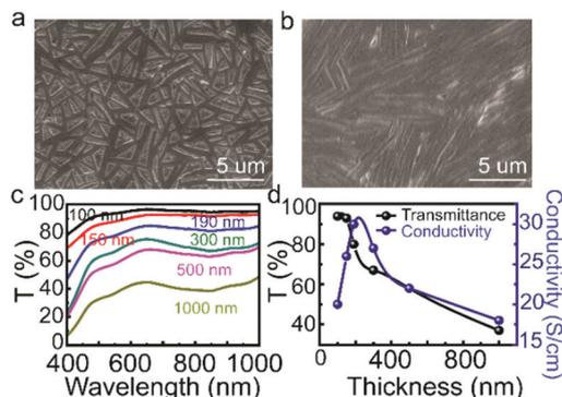
**Fig. 3** (a and b) The SEM images of the TTF-TCNQ film with different thicknesses (100 nm for a and 300 nm for b). (c) The transmittance of the TTF-TCNQ film with different thicknesses (from 100 nm to 1000 nm). (d) The thickness dependent transmittance at 550 nm and the thickness dependent conductivities of the TTF-TCNQ film.
