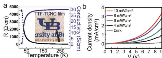
**Fig. 4** (a) The temperature-dependent resistivity and conductivity of the TTF-TCNQ film with optimum transparency and conductivity. Inset: the photograph of the TTF-TCNQ film. (b) The current density-voltage curves of the all-organic photodetector under light illumination with different intensities.
