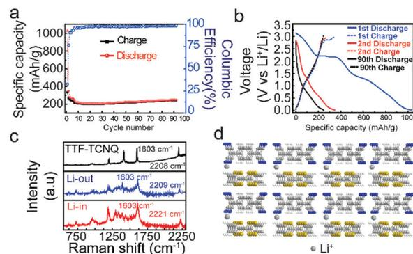
**Fig. 5** (a) Cycle performance of the lithium-ion battery using TTF-TCNQ as the anode. (b) The discharging/charging curves of the lithium-ion battery using TTF-TCNQ as the anode. (c) The Raman spectra of the TTF-TCNQ film at different stages of Li intercalation. (d) The schematic diagram of the Li ion storage.
