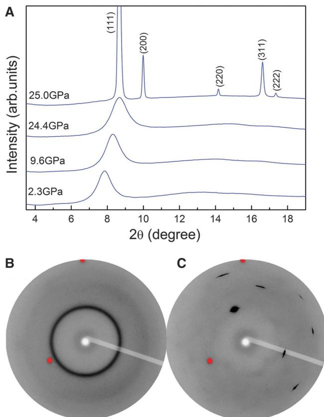
**Fig. 3.** The 2D XRD image of the fcc single crystal quenched to ambient pressure. The image is indexed as a  $Z$ - $[\bar{1}\bar{1}0]$  zone-axis pattern with  $\pm 5^\circ$  rotation of the  $\omega$  axis. The relationship between the crystallographic orientation and ribbon geometry is shown in the schematic illustration.
