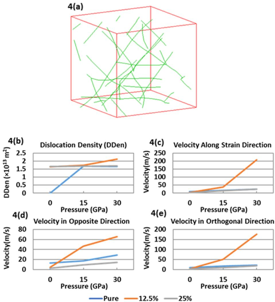
FIG. 4. (a) Initial dislocation setup for  $1 \times 1 \times 1 \mu\text{m}^3$  cubic FCC Ni metal in ParaDiS. (b) Dislocation density of S doped Ni under different pressures in ParaDiS simulation. (c) The dislocation velocity component contributing to strain rate. (d) The dislocation velocity component in the opposite direction. (e) The dislocation velocity component in the orthogonal direction.
