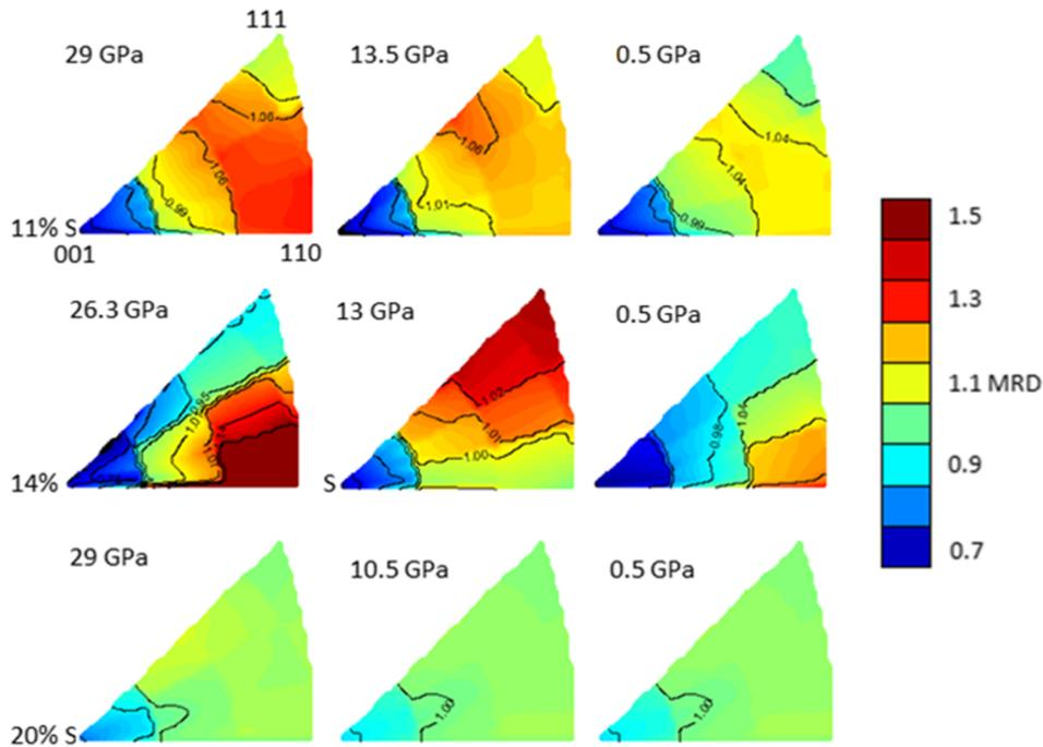
FIG. 2. Inverse pole figures of S doped nickel metal samples with 11 at.%, 14 at.%, and 20 at.% S concentrations along ND under decompression shear stress.
