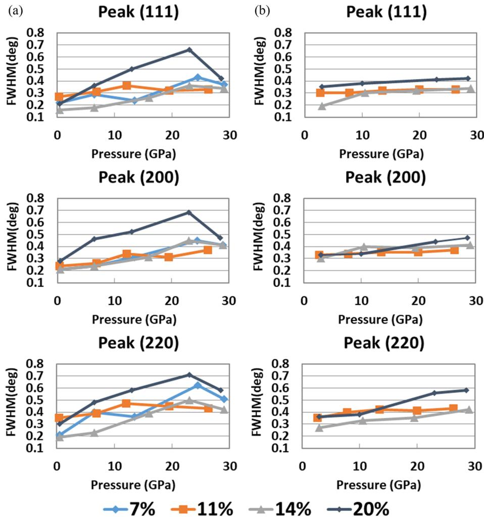
FIG. 3. The peak broadening of nickel in S doped Ni samples under compression and decompression shear stress. The full width at half maximum (FWHM) is used. The curves are offset for clarity. For the FWHM determination, the signal is integrated over 10 degrees around the compression direction. (a) represents the compression data, whereas (b) represents the decompression data.
