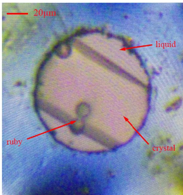
Fig. 1. A view of the DAC high-pressure chamber with the pressure-induced single crystal of *o*-xylene. Three ruby balls for pressure calibration are located in the chamber.
