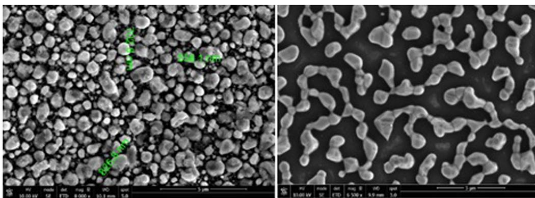
Fig. 7. Scanning electron micrographs of amorphous Co treated at 900 °C (a) without the magnetic field and (b) within 6.8 T magnetic field.
