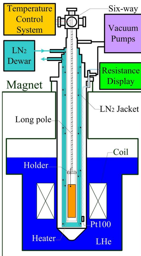
Fig. 1. Schematic of the furnace system within a cold bore superconducting magnet, showing the five-tube shielding system and its connections to other important components.
