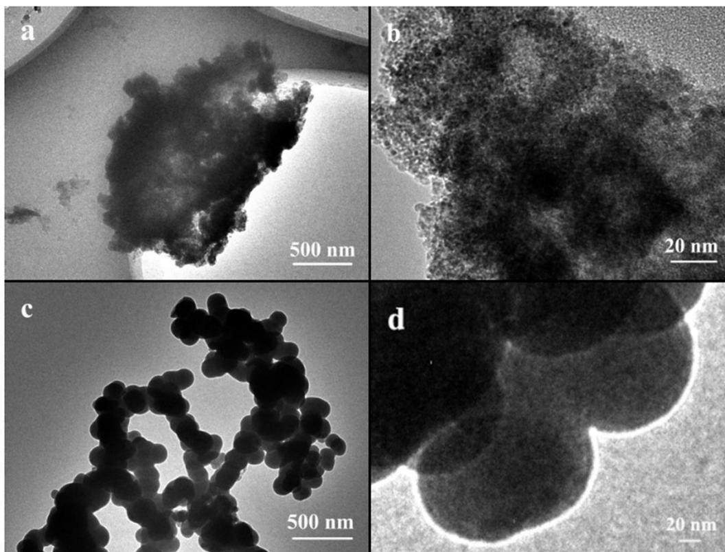
Fig. 6. Transmission electron micrographs of the products prepared (a, b) without the magnetic field and (c, d) within 15 T magnetic field.
