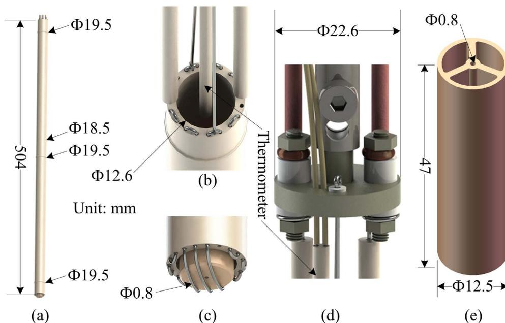
Fig. 2. Details of the heater. (a) Design picture of the long corundum tube, with detail of its (b) top and (c) bottom regions, (d) picture showing connections with the holder, and (e) three-dimensional schematic of corundum tube designed for samples.
