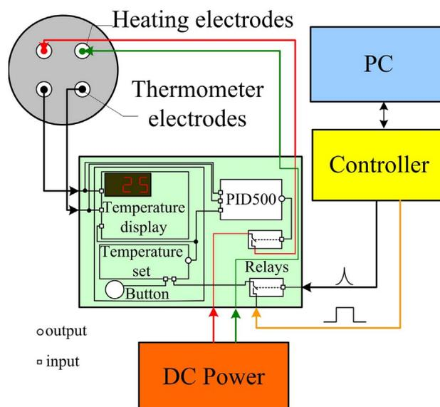
Fig. 4. Schematic of temperature controlling system.
