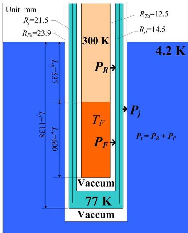
Fig. 5. Schematic of radiation analysis.
