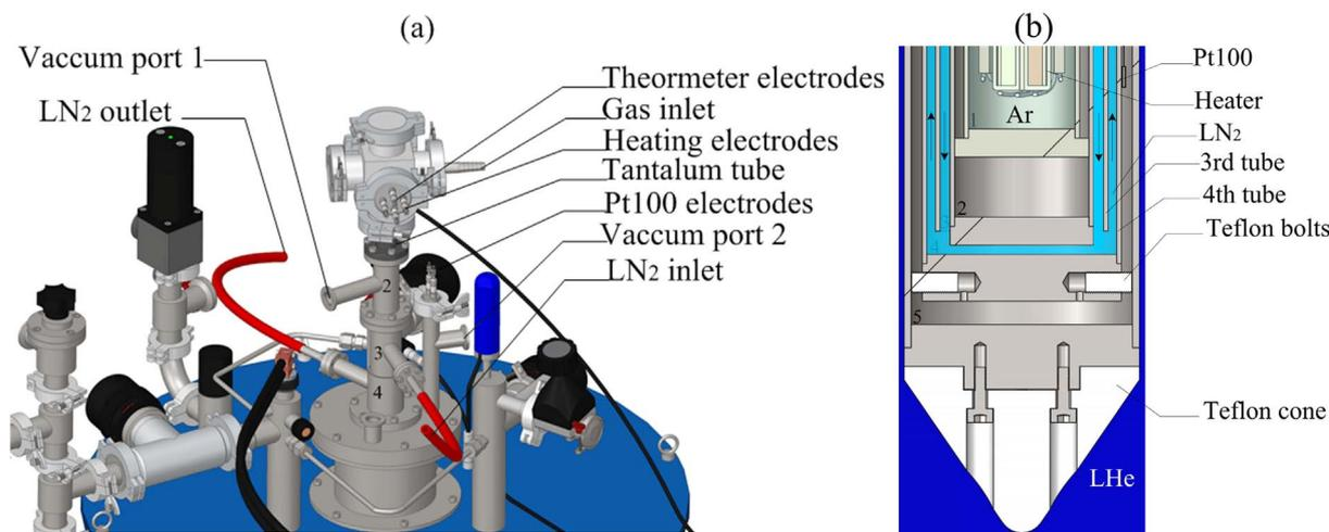
Fig. 3. Detail of the (a) top and (b) bottom of the furnace chamber. The former is a three-dimensional design image and the latter is a sectional drawing.
