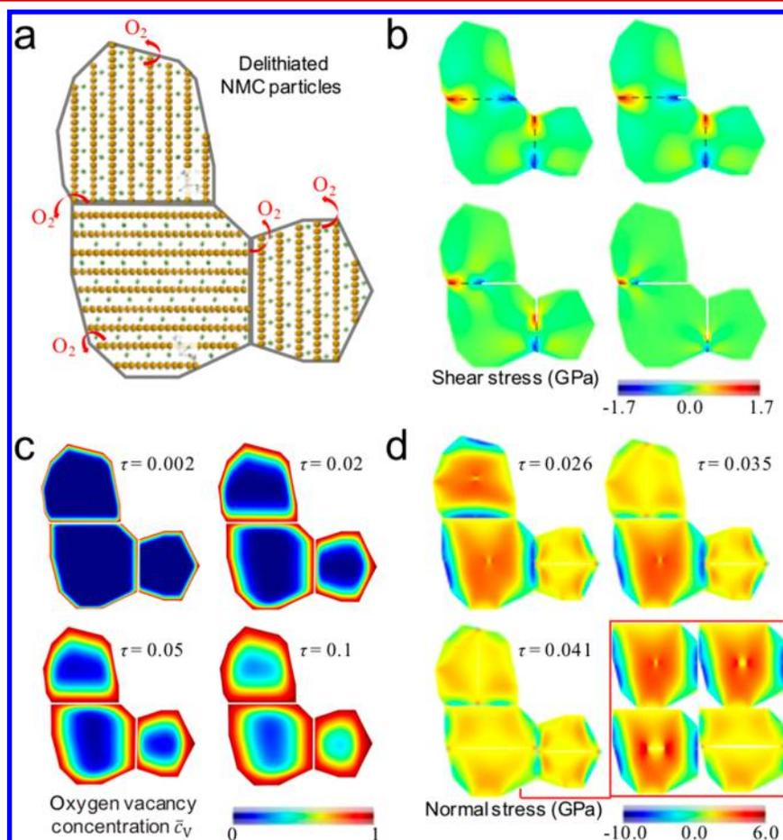
**Figure 5.** (a) Finite element modeling (FEM) model consisting of multiple NMC grains of different orientations. (b) Evolution of shear stress along the grain boundaries and associated intergranular cracks induced by the phase transformation of NMC. (c) Profile of the oxygen vacancies, and (d) nucleation and propagation of intragranular cracks induced by oxygen release in NMC. The inset in part d shows the initiation and rapid propagation of the intragranular crack in the lower left NMC grain.
