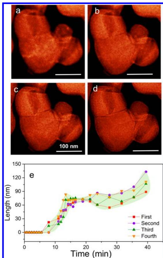
**Figure 2.** Selected Z-contrast scanning transmission electron microscopy (STEM) images to represent the evolution of a typical intergranular crack upon thermal activation: (a) 0, (b) 12, (c) 26, and (d) 40 min. (e) Evolution of crack length as a function of time, where four cracks (indicated by arrows in Figure S2) were independently measured and are presented here.
