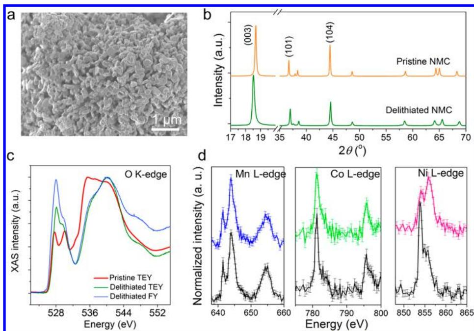
**Figure 1.** (a) SEM image of the pristine NMC material. (b) XRD patterns of pristine and delithiated NMC materials. (c) O K-edge XAS collected in the TEY and FY modes for pristine (red/TEY) and delithiated (green/TEY and blue/FY) NMC materials. (d) TM L-edge XRS of pristine (bottom) and delithiated (top) NMC materials. The error bars were calculated based on the standard deviations of six repeated data acquisitions under identical experimental conditions.
