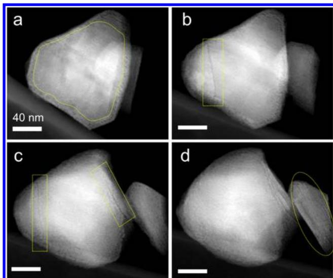
**Figure 4.** (a–d) STEM images for the same two particles taken from different directions to exhibit the 3D view of delithiated NMC particles after *in situ* heating on a TEM grid. The regions enclosed by yellow dashed curves display intragranular cracks. The scale bars are 40 nm for all images.
