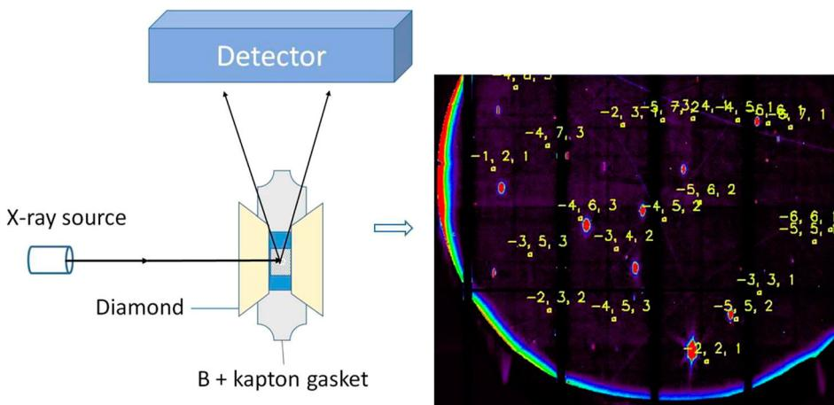
**Figure 2.** Left: Experimental set-up of high pressure Laue X-ray microdiffraction. Right: indexed Laue pattern of one WC grain embedded in 3 nm nickel.
