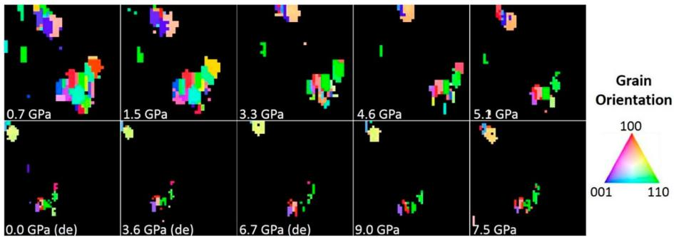
**Figure 4.** 2D crystal orientation maps of WC marker embedded in 3 nm nickel at different pressures.
