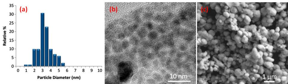
**Figure 1.** (a) Particle size distribution of 3 nm nickel (Image courtesy of nanoComposix); (b) TEM image of 3 nm nickel; (c) SEM image of 500 nm nickel.
