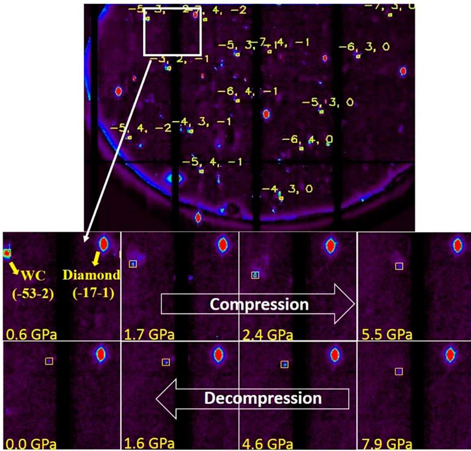
**Figure 5.** Evolutions of a tracked WC spot (-53-2) embedded in 500 nm nickel at different pressures. The centroid coordinates of all cutoffs are 414 and 92 with a zoom factor of 2.
