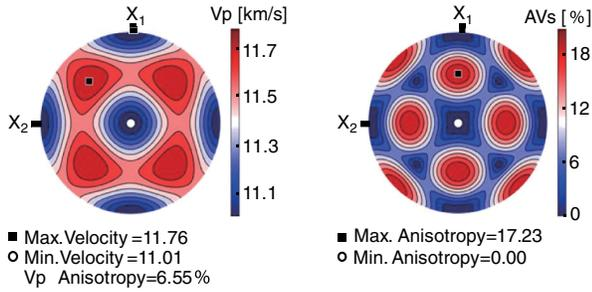
FIG. 4. Stereographic projections of the calculated  $P$ -wave velocity  $V_P$  (in km/s) and  $S$ -wave anisotropy  $AV_S$  (in %) for  $Fm-3m$   $\text{FeO}_2\text{He}$  at 135 GPa and 3000 K. The coordinate axes are  $X_1 = [100]$ ,  $X_2 = [010]$ ,  $X_3 = [001]$ . The black square and white circle in each plot indicate the crystallographic directions of the maximum and minimum values, respectively.
