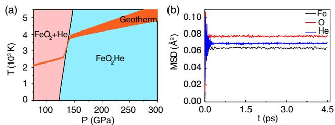
FIG. 2. (a) Pressure-temperature ( $P$ - $T$ ) phase diagram showing the stability field of  $Fm\text{-}3m$   $\text{FeO}_2\text{He}$  and its boundary with the decomposition products  $\text{FeO}_2 + \text{He}$ . Also shown is the geotherm indicating the  $P$ - $T$  profile in Earth's interior. (b) Calculated mean-square-deviation (MSD) of the atomic positions of  $Fm\text{-}3m$   $\text{FeO}_2\text{He}$  at 135 GPa and 3000 K.
