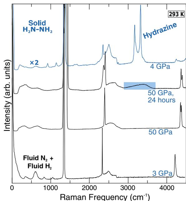
FIG. 4. Raman spectra on compression of a 50 mol%  $\text{H}_2$  composition demonstrating the time-dependent chemical reaction of  $\text{N}_2$  and  $\text{H}_2$  above 50 GPa. The blue shaded region indicates the formation of N–H bonds. The blue spectrum shows the recovery of hydrazine on decompression to 4 GPa. For a comparison between these data and Ref. [20], see Figs. S14 and S15 [36].
