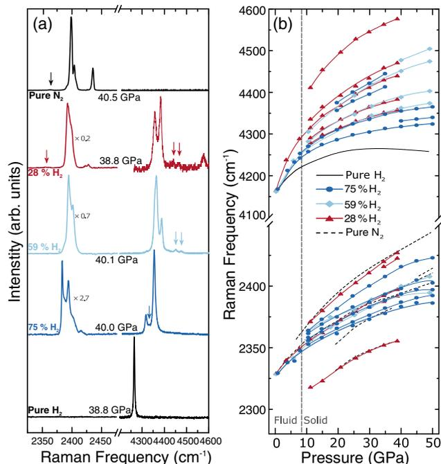
FIG. 2. (a) Evolution of the Raman spectra with composition in the solid state at around 40 GPa for the nitrogen-hydrogen compositions of 28, 59, and 75 mol % H<sub>2</sub>. The pure species are included for comparison in black. (b) Raman frequency vs pressure plots corresponding to the data shown in (a). Solid and dashed black lines correspond to pure H<sub>2</sub> and pure N<sub>2</sub>, respectively. Arrows indicate weak Raman bands.
