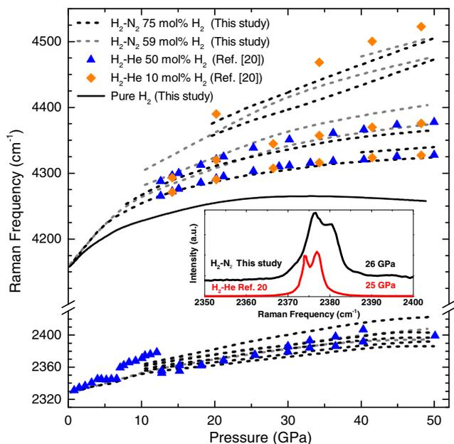
FIG. 3. A comparison of the Raman frequencies as a function of pressure between our data on  $\text{H}_2\text{-N}_2$  mixtures (dashed lines), pure  $\text{H}_2$  (black line), and the  $\text{H}_2\text{-He}$  compound (known as “ $S_2$ ”) reported in Ref. [20] (symbols). (Inset) Comparison between “H-He” vibrons from Ref. [20] and the  $\text{N}_2$  vibrons from a 3:2  $\text{H}_2\text{-N}_2$  mixture.
