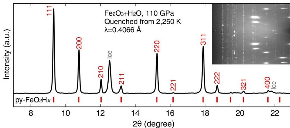
**Figure 2. X-ray diffraction pattern of reaction product of Fe<sub>2</sub>O<sub>3</sub> and water.** The sample was compressed to 110 GPa, heated to 2,250 K and quenched to 300K. py: pyrite structured
