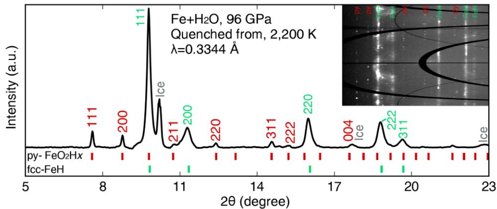
**Figure 1. X-ray diffraction pattern of reaction products of iron and water.** Iron powder was compressed in H<sub>2</sub>O to 96 GPa, heated up to 2,200 K for 5 minutes, and quenched to 300 K. The pattern was composed of the Py-phase ( $a=4.370(3)$  Å), the quenchable high-temperature f.c.c phase[43] of FeH ( $a=3.397(4)$  Å), and excess ice VII. Inset figure is the caked diffraction pattern, showing the coexistence of the Py-phase (dotted reflections) and FeH (continuous reflections).
