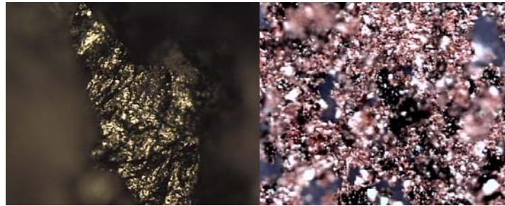
Figure 2. Optical photos of (a) synthesized  $\gamma\text{-B}_{28}$  sample recovered from 12 GPa and 1500°C and (b) grinded  $\gamma\text{-B}_{28}$  sample.
