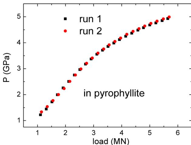
FIG. 6. The load-pressure curves during decompression in two different experiments using pyrophyllite as a transmitting medium.
