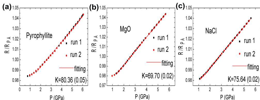
FIG. 2. The relative resistance of manganin as a function of the pressure in three different solid media.
