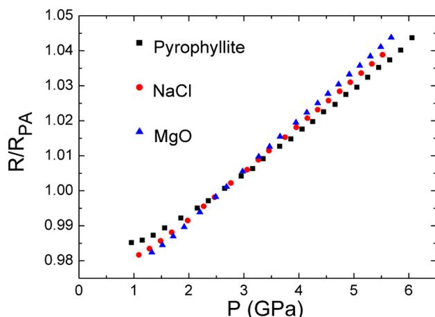
FIG. 3. Different responses of the manganin's resistance to the pressure in various PTM.
