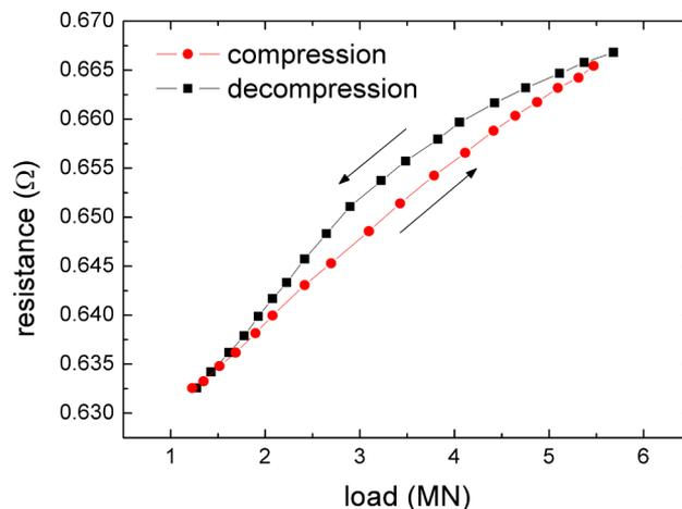
FIG. 4. Resistance of manganin in the compression and decompression processes.
