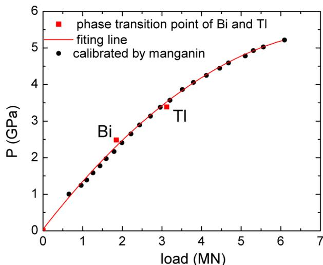
FIG. 5. The load-pressure curves calibrated by manganin and the phase transition points of Bi and Ti.
