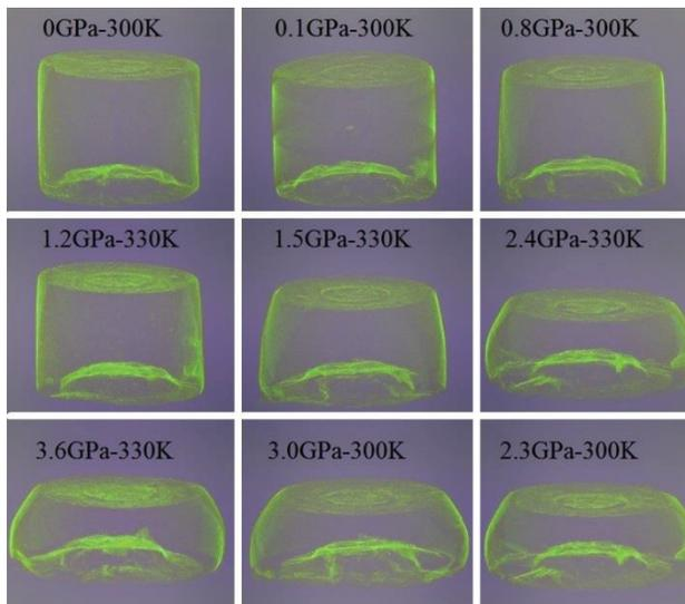
**FIGURE 3.** 3D images for the gallium as a function of pressure and temperature.
