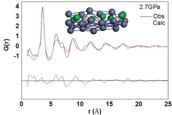
**FIGURE 10.** Experiment data from Yb-based metallic glass (black line) and calculated data using PDFFIT (pink line). Below is plotted a difference curve.
