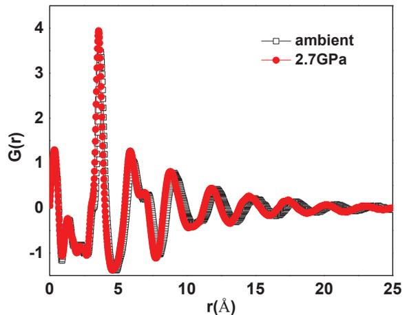
FIGURE 8.  $G(r)$  of Yb-based metallic glass under ambient pressure and 2.7GPa.
