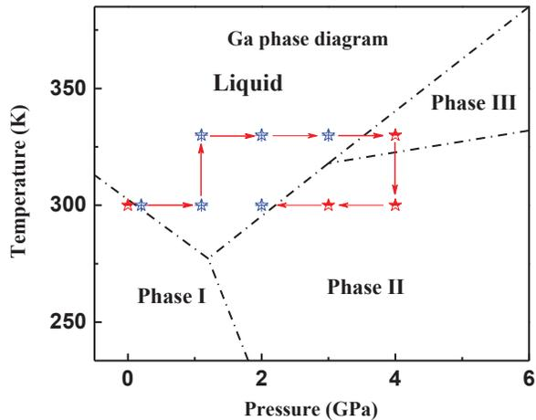
**FIGURE 2.** Pressure-temperature paths for gallium in X-ray microtomography. Phase diagram of gallium is cited from Ref. 6.
