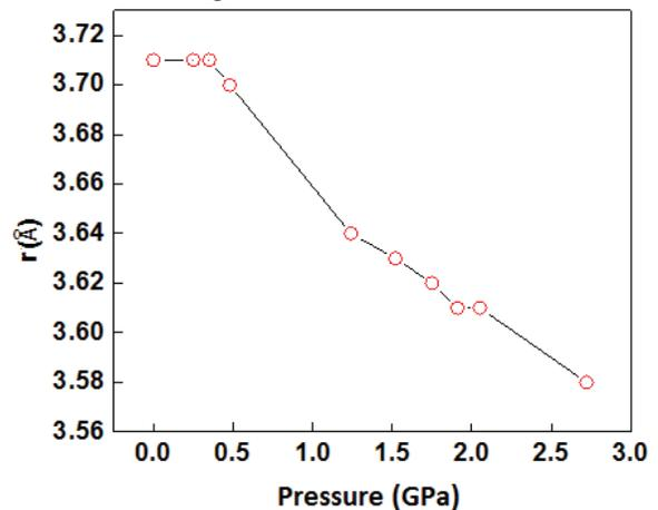
FIGURE 9. Relative distance between nearest-neighbor atoms as a function of pressure at ambient temperature.
