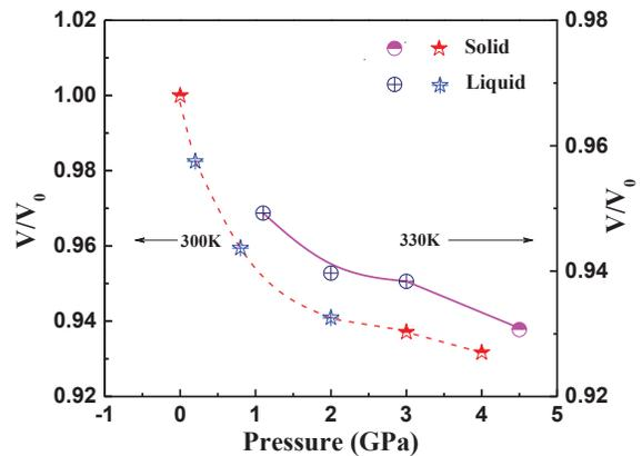
**FIGURE 5.** Relative volume  $V/V_0$  of the gallium as a function of pressure and temperature at 300K and 330 K.
