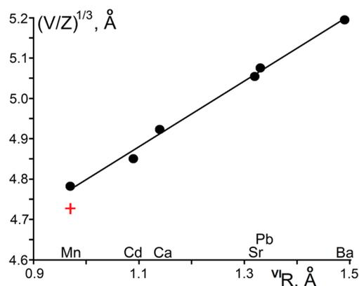
**Figure 3.** Correlation between the cubic roots of the formula volumes of  $\text{MSb}_2\text{O}_6$  and the octahedral radii of  $\text{M}^{2+}$  cations:<sup>50</sup> (filled circles)  $\text{PbSb}_2\text{O}_6$ -type phases and (cross) stable  $\text{MnSb}_2\text{O}_6$  phase.
