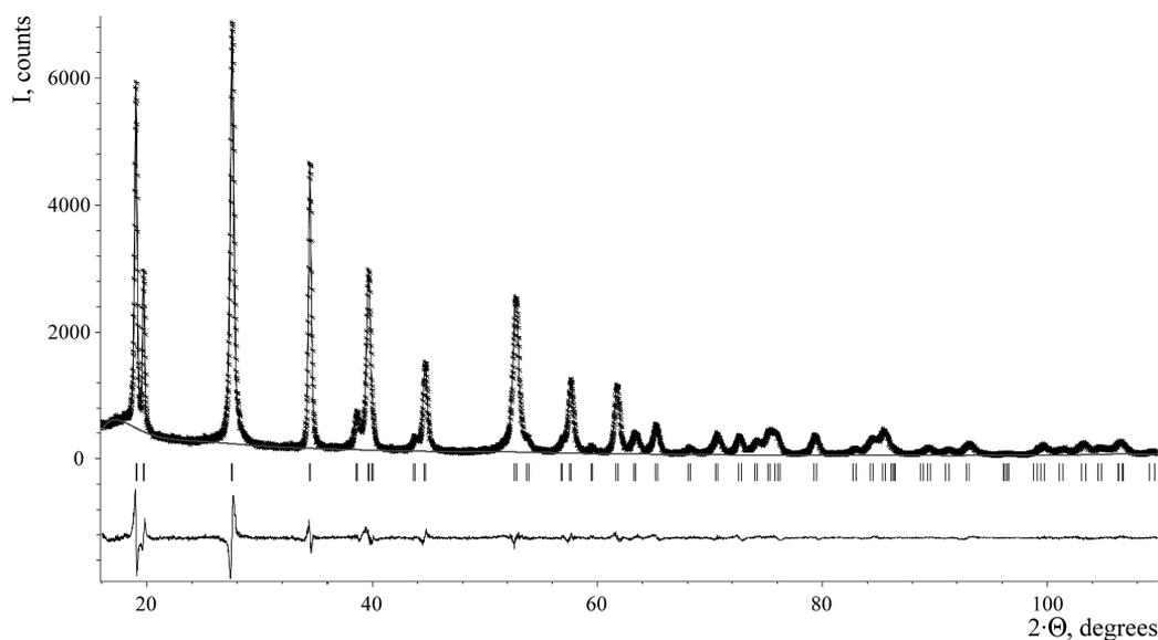
**Figure 2.** XRD pattern of  $\text{MnSb}_2\text{O}_6$ , where the points are the experimental data, the line the calculated pattern, the line at the bottom the difference profile, and the vertical bars the peak positions.
