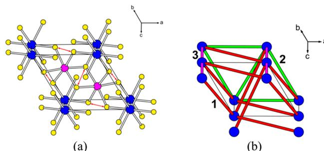
**Figure 6.** (a) Perspective view of the crystal structure and (b) spin exchange paths in  $\text{MnSb}_2\text{O}_6$  where the blue, pink, and yellow circles represent Mn, Sb, and O atoms, respectively, and the numbers 1, 2, and 3 indicate the spin exchange paths  $J_1$ ,  $J_2$ , and  $J_3$ , respectively.
