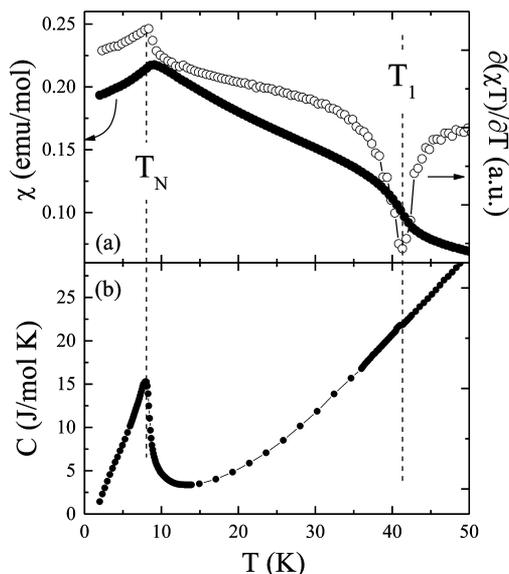
**Figure 5.** (a) Temperature dependence of the magnetic susceptibility at  $B = 0.01$  T, of the magnetic specific heat  $\partial(\chi T)/\partial T$ , and (b) of the specific heat at  $B = 0$  T highlighting two different anomalies at  $T_N$  and  $T_1$ .
