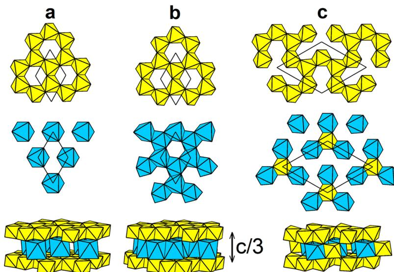
**Figure 1.** Polyhedral presentation of the crystal structures of (a)  $\text{CaSb}_2\text{O}_6$  ( $P\bar{3}1m$ ),<sup>45</sup> (b)  $\text{NaSbO}_3$  ( $\text{Na}_2\text{Sb}_2\text{O}_6$ ,  $R\bar{3}$ ),<sup>46</sup> and (c)  $\text{MnSb}_2\text{O}_6$  ( $P321$ ).<sup>42</sup> (Top row) Layer of  $\text{SbO}_6$  octahedra, (middle row)  $\text{MO}_6$  octahedra ( $M = \text{Ca}^{2+}$ ,  $\text{Na}^+$ , or  $\text{Mn}^{2+}$ ), and (bottom row) layer stacking pattern.
