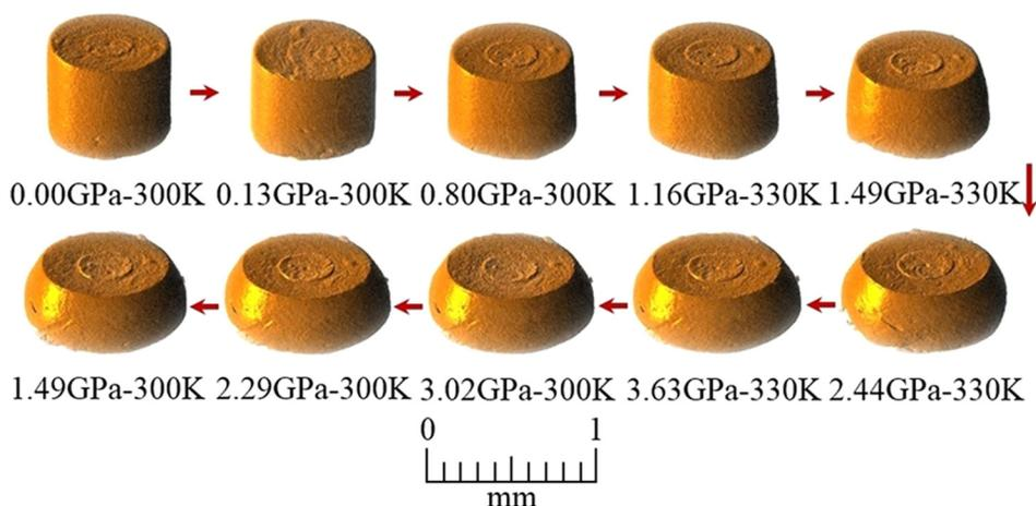
FIG. 4. Reconstructed 3D images for the gallium as a function of pressure and temperature. The order follows experimental P-T path in Fig. 2.
