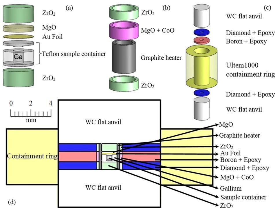
FIG. 1. Illustrations of Drickamer cell for the microtomography measurements. (a)–(c) The detailed cell assemblage. (d) Scaled view of section of Drickamer cell used in this study.
