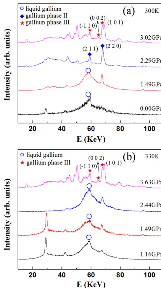
FIG. 3. Selected typical EDXRD patterns of Ga as a function of pressure at (a) 300 K and (b) 330 K.
