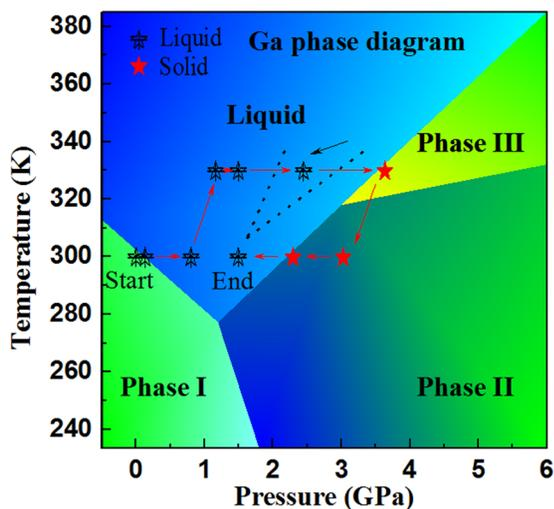
FIG. 2. Pressure-temperature paths for gallium in X-ray microtomography and EDXRD experiments. Phase diagram of gallium is cited from Ref. 6. The dotted lines outline a possible liquid-liquid transition region.
