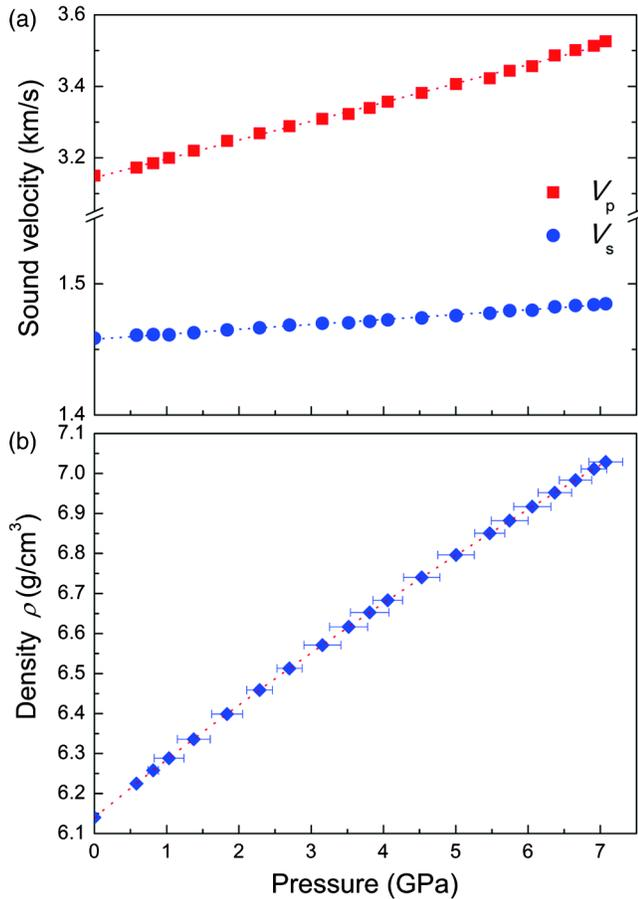
FIG. 2 (color online). Density measurement of L62 BMG using integrated ultrasonic sound velocity, x-ray radiography, and XRD measurements. (a) The sound velocities of the compression wave ( $V_p$ ) and shear wave ( $V_s$ ) as a function of pressure up to 7.1 GPa. (b) The density as a function of pressure obtained by calculation from ultrasonic sound velocities. The dotted line represents the fitting of density data using the third-order BM-EOS.
