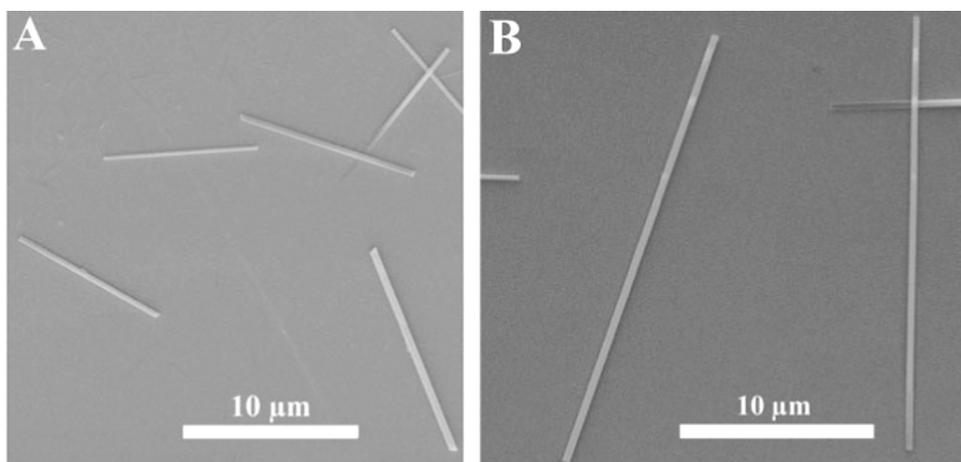
Fig. 5. SEM images of as-grown  $C_{60}$ \**m*-xylene solvate nanorods. [28,29] (Reprinted with permission from Wang et al. [29]).
