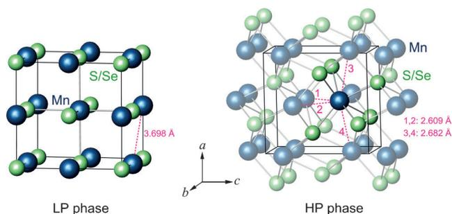
**Figure 2.** Illustration of the crystal structures for the LP ( $Pm\bar{3}m$ ) and HP ( $Pnma$ ) phases of MnS and MnSe (Mn, blue; S/Se, cyan). The distorted Mn(S,Se)<sub>6</sub> octahedron is highlighted in the HP structure and the shortest or the near-shortest Mn–Mn bond lengths are shown by dashed lines. The schematic bond-length values are taken from the MnS structures at ambient conditions and 31.2 GPa, respectively.
