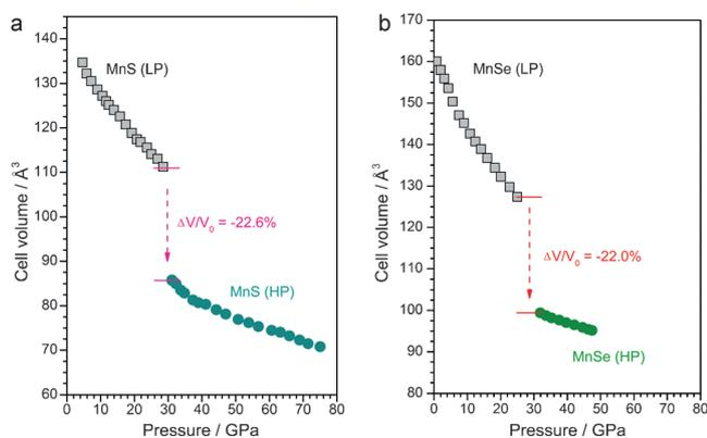
**Figure 1.** Experimental cell volumes as a function of applied pressure for the LP and HP phases of a) MnS and b) MnSe. The fitting of the  $P$ - $V$  data according to the third-order Birch–Murnaghan equation-of-state functions gives bulk modulus  $B_0$  (LP) = 72,  $B_0$  (HP) = 80 GPa for MnS, and  $B_0$  (LP) = 68,  $B_0$  (HP) = 218 GPa for MnSe, respectively.
