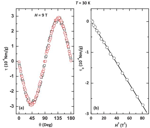
**Figure 3.** (a) Typical angular  $\theta$  dependent torque  $\tau$  at temperature  $T = 30$  K with a magnetic field  $H = 9$  T. (b)  $\tau_0$  versus  $H^2$  at  $T = 30$  K.
