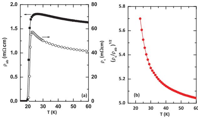
**Figure 1.** (a) Temperature  $T$  dependent in-plane and out-of-plane resistivity data,  $\rho_{ab}$  (left axis),  $\rho_c$  (right axis). (b)  $T$  dependent resistivity anisotropy  $(\rho_c/\rho_{ab})^{1/2}$ .
