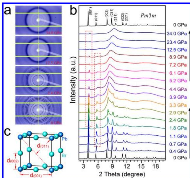
**Figure 1.** Synchrotron XRD patterns of MAPbBr<sub>3</sub> obtained during compression up to 34.0 GPa and decompression: (a) The raw 2D XRD images and (b) integrated 1D XRD profiles. The XRD pattern after decompression can be indexed with the same crystal structure (space group  $Pm\bar{3}m$ ) from the pristine materials. (c) Illustration of the representative interplanar distances in MAPbBr<sub>3</sub> lattice (Only Pb and Br atoms are drawn for clarity).
