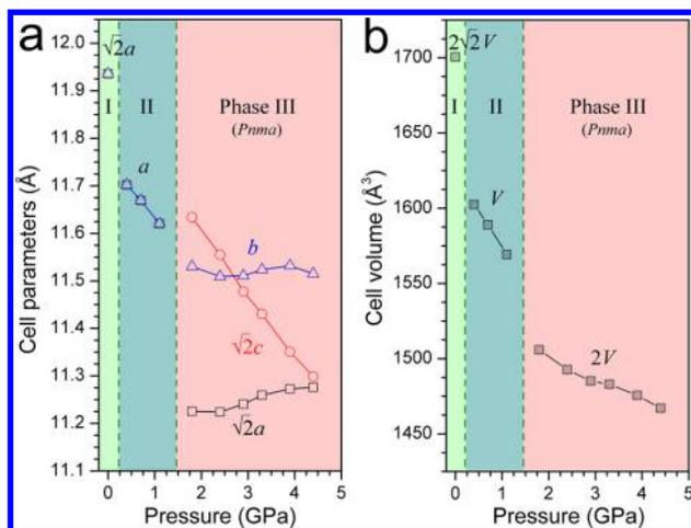
**Figure 3.** Unit cell parameters (a) and volume evolutions (b) of MAPbBr<sub>3</sub> as a function of pressure at room temperature. Space group of I: cubic, *Pm* $\bar{3}$ *m*; II: cubic, *Im* $\bar{3}$ ; III: orthorhombic, *Pnma*.
