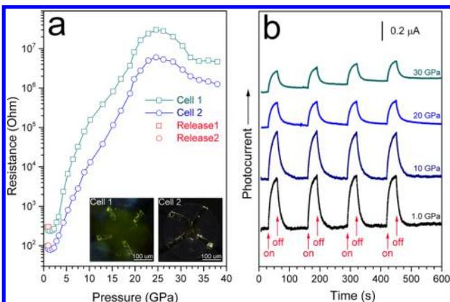
**Figure 6.** Electrical resistance (a) and photocurrent (b) of MAPbBr<sub>3</sub> as a function of pressure. The insert in panel (a) displays microphotographs of the samples in two DACs with Au probes.
