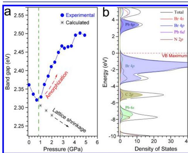
**Figure 5.** Derived band-gaps of MAPbBr<sub>3</sub> as a function of pressure (a) and calculated partial density of states from each element in the compound (b).
