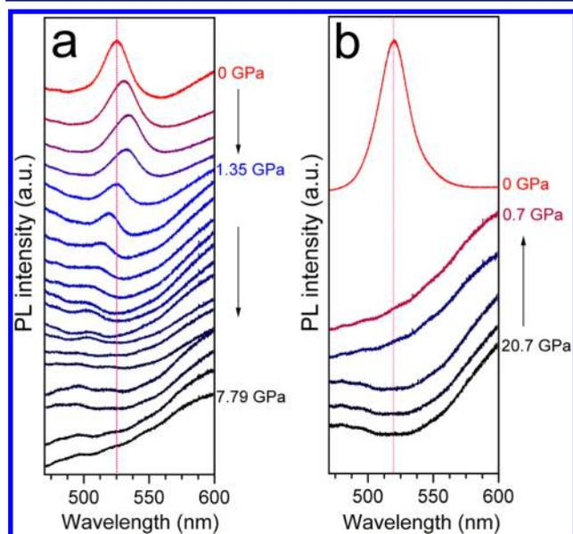
**Figure 4.** Room temperature photoluminescence spectra of MAPbBr<sub>3</sub> as a function of pressure during compression (a) and decompression (b). A 325 nm and 3 mW laser was used for irradiation.
