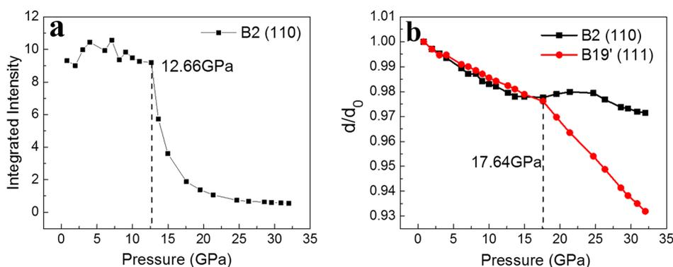
FIG. 4. Compression behavior of the NiTi matrix. (a) Intensity of NiTi-B2 (110) reflection versus pressure. From 14.7 GPa to 17.4 GPa, a fast reduction in the diffraction intensity of the B2(110) reflection is observed. (b) The relative d-spacing of B2 (110) and B19' (111) reflections versus pressure. Beyond 17.4 GPa, the B19' (111) lattice decreases more rapidly than the low-pressure compression rate, while the B2 (110) lattice shows a similar anomalous compression behavior to the Nb nano-rods.
