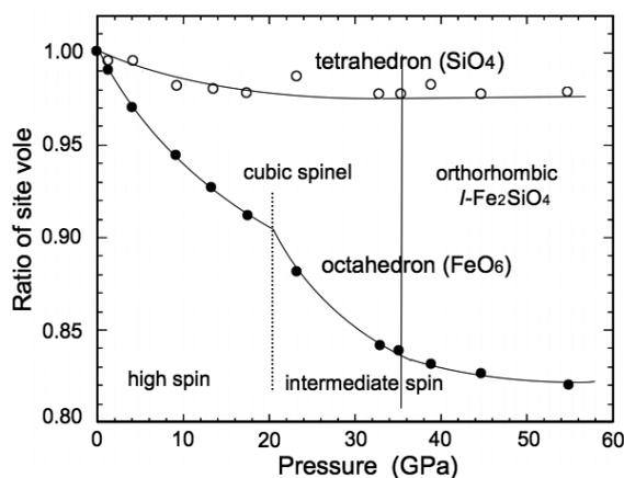
**FIGURE 3.** Average bond length ratio of tetrahedral and octahedral sites of Fe<sub>2</sub>SiO<sub>4</sub> spinel. Bond lengths were obtained from the Rietveld profile fitting method. Error is smaller than the symbol mark. The Fe-O bond length in the octahedral site confirms the two different compression regimes at 20 GPa.
