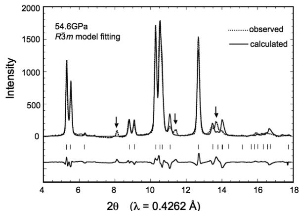
**FIGURE 5.** Rietveld profile fitting of the initial structure model of rhombohedral Fe<sub>2</sub>SiO<sub>4</sub> to the data obtained at 54.6 GPa. The rhombohedral structure model (space group  $R\bar{3}m$ ) is simply derived from a distortion along the  $\langle 111 \rangle$  direction of the spinel structure. Peaks indicated by the arrows are not indexed.
