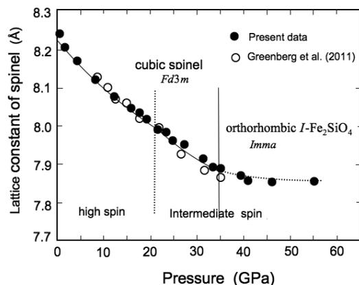
FIGURE 2. There are two distinct compression regimes indicating the boundary at about 20 GPa. This behavior is a little higher pressure than the HS-to-IS transition of 17 GPa observed by XES. The data of Greenberg et al. (2011) are also presented. The dotted curve represents the lattice parameter of the residual spinel coexist with *I*-Fe<sub>2</sub>SiO<sub>4</sub>. The observed error is smaller than the data point.
