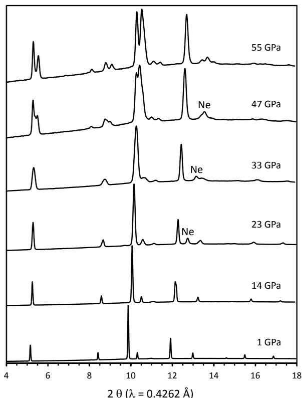
FIGURE 1. Selected X-ray diffraction patterns of Fe<sub>2</sub>SiO<sub>4</sub> taken with increasing pressure at ambient temperature. The high-pressure phase was found above 38.8 GPa and observed up to 56.6 GPa.
