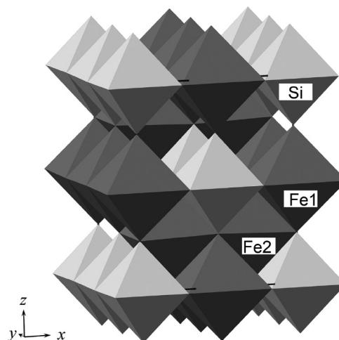
**FIGURE 8.** There are two distinct octahedral Fe sites, Fe1 and Fe2. Si is also located at the site of octahedral coordination. Fe1 and Fe2 octahedra create layers parallel to the (101) and (011) planes, respectively. SiO<sub>6</sub> octahedra make an array in the direction of  $\langle 010 \rangle$ .
