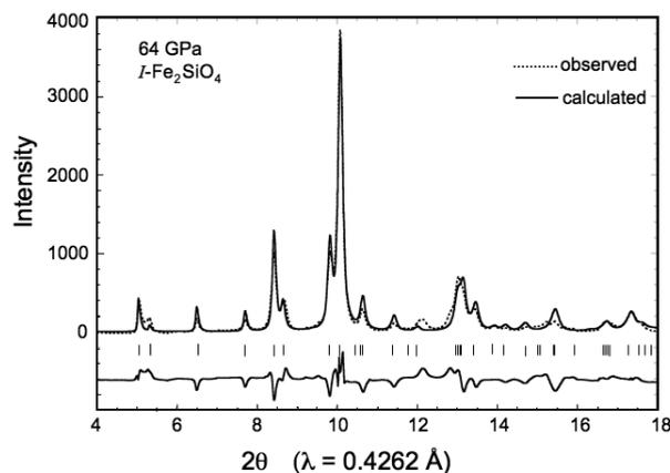
**FIGURE 7.** Rietveld profile fitting of diffraction data obtained at 64 GPa. Rietveld profile fitting was carried out in consideration of two-phase mixture of  $I$ -Fe<sub>2</sub>SiO<sub>4</sub> and spinel. No spinel peaks are, however, detected and only a single phase of  $I$ -Fe<sub>2</sub>SiO<sub>4</sub> is observed. Vertical bars indicate peak positions of the  $I$ -Fe<sub>2</sub>SiO<sub>4</sub>.
