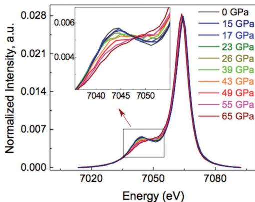
**FIGURE 10.** FeK $\beta$  X-ray emission spectra with increasing pressure up to 64.8 GPa. The inset shows the expanded K $\beta$ ' spectra, indicating an intermediate spin transition. The spin transition occurs at  $\sim$ 17 GPa. (Color online.)
