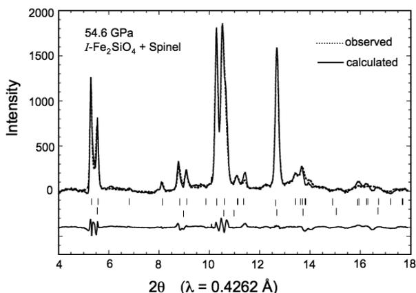
**FIGURE 6.** Rietveld profile fitting of diffraction data obtained at 54.6 GPa, assuming a two-phase mixture of orthorhombic Fe<sub>2</sub>SiO<sub>4</sub> and spinel. Upper and lower vertical bars indicate peak positions for orthorhombic Fe<sub>2</sub>SiO<sub>4</sub> and spinel, respectively.
