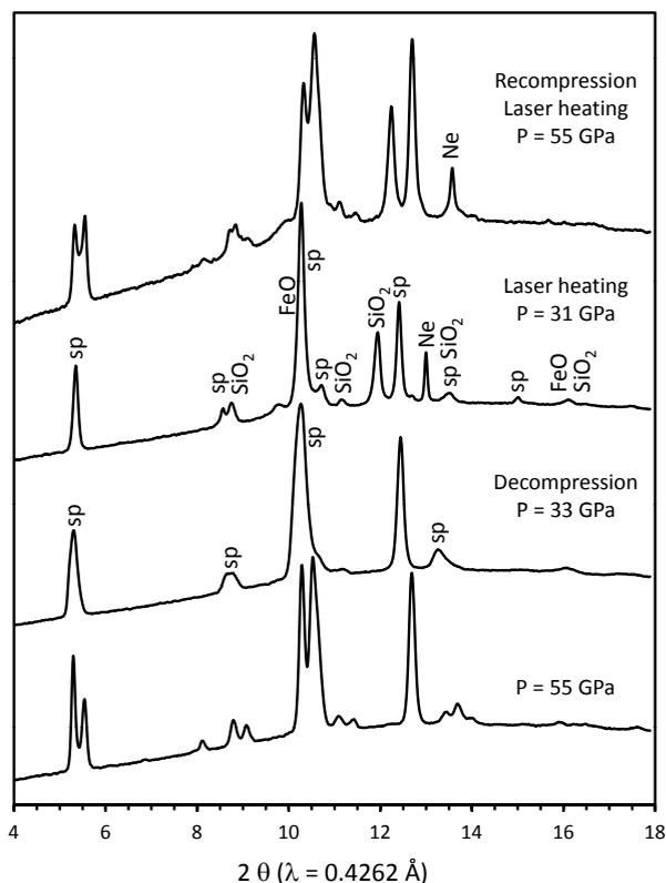
**FIGURE 4.** The decompression experiment confirms a reversible transition between cubic and orthorhombic phases. Subsequent laser heating at 1500 K and 31 GPa reveals decomposition from spinel to rhombohedral FeO and SiO<sub>2</sub> stishovite.
