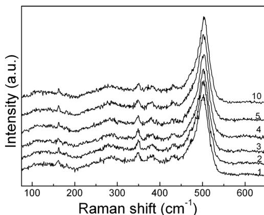
FIG. 4. A series of Raman spectra collected at 1 atm in an indentation with a collection time of 1 s for each spectrum using a 24 mW laser. The testing region was not exposed to the laser between each collection. The number labeled above each spectrum is the sequence of the spectrum.
