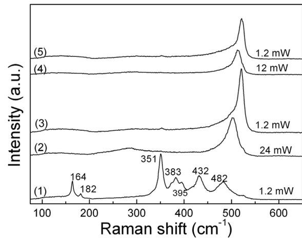
FIG. 3. A series of Raman spectra collected at 1 atm in an indentation using different laser powers: 1.2 mW (1), 24 mW (2), 1.2 mW (3), 12 mW (4), and 1.2 mW (5). The collection time was set to 1 s for the 24 mW and 12 mW measurements, and 20 s for the 1.2 mW measurements.
