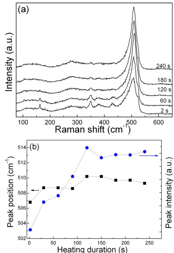
FIG. 5. (a) A series of Raman spectra collected at 1 atm in an indentation with a collection time of 2 s during continuous laser annealing at 24 mW. The number above each spectrum is the annealing duration when the spectrum was collected. (b) The peak position (black squares) and peak intensity (blue dots) as functions of the annealing time. The peaks are fit with Voigt functions after linear background subtraction.
