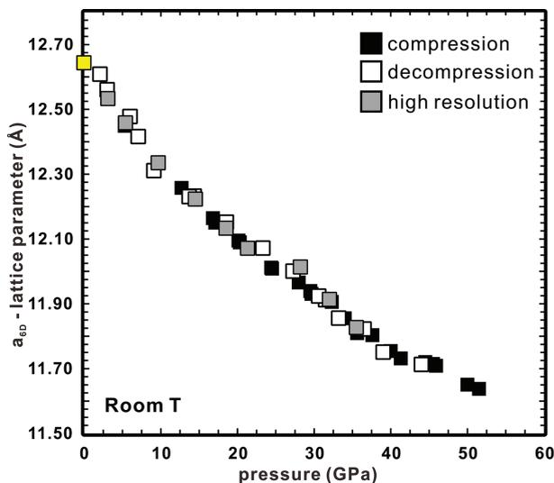
**FIGURE 3.** Variation of the lattice parameter as function of pressure: yellow square, ambient-pressure value (Bindi et al. 2011); black and white squares indicate lattice parameter determined, respectively, from compression and decompression experiments; gray squares indicate experiments at higher resolution. (Color online.)
