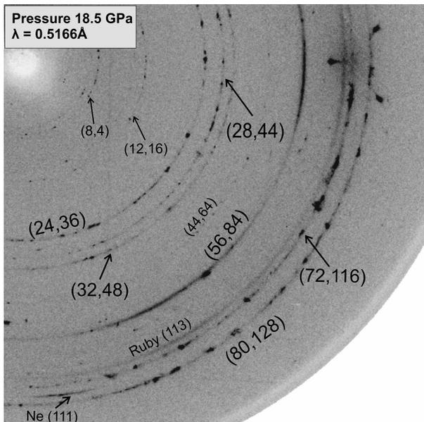
**FIGURE 1.** Representative X-ray diffraction pattern of  $i\text{-Al}_{63}\text{Cu}_{24}\text{Fe}_{13}$  collected at  $P = 18.5$  GPa. Diffraction rings and weak single spots are typical features of the collected patterns. The Debye-Scherrer rings are labeled as in case of QCs using the two-integer indexes by Janot (1994). The diffraction patterns were processed using Fit2D (Hammersley 1998) and Peakfit software.
