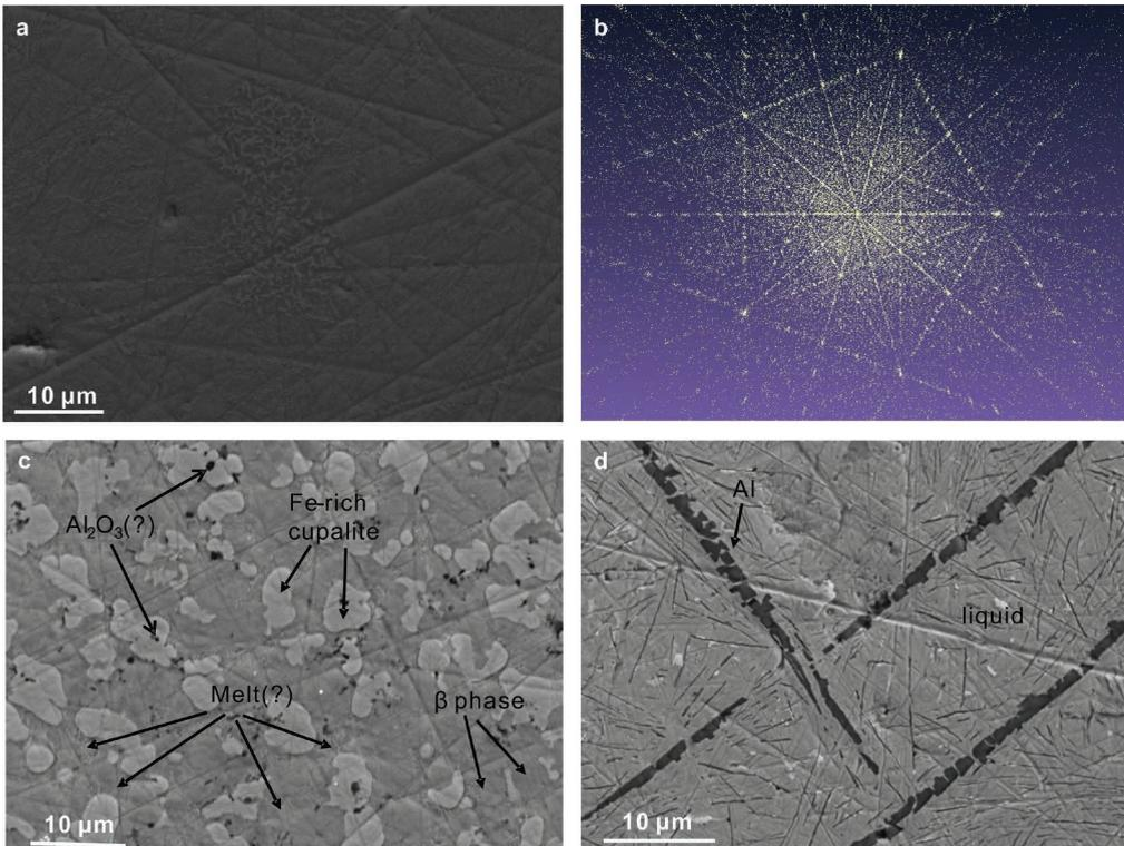
**FIGURE 6.** Back-scattered electron (BSE) images of the recovered sample from runs at 21 GPa. (a) Run at 1673 K showing the presence of i-QC also confirmed by the fivefold symmetry in (b) using single-crystal X-ray diffraction. (c) Recovered sample from 21 GPa and 1773 K and (d) 1973 K, respectively. (Color online.)
