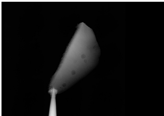
Movie S1. FIBed section of RSES 61-18.8, imaged by transmission X-ray microscopy. The section is rotated around a tungsten needle attached to one end. Several fully enclosed inclusions are visible. Fig. 1 of the main text points out the carbonaceous phases. Imaging is by Crystal Shi (Department of Earth, Energy, and Environmental Sciences, Stanford University, Stanford, CA).
