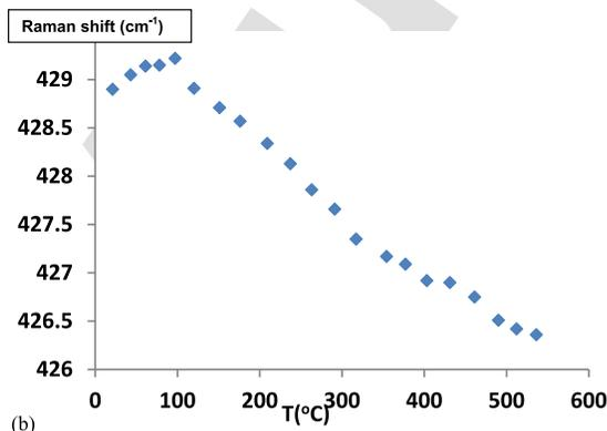
FIG. 5. Temperature dependencies of the Raman modes of  $\text{Sr}_2\text{MgTeO}_6$ . Discontinuity and slope change are observed around 100 °C and 300 °C. The inset shows results of repeated experiment.
