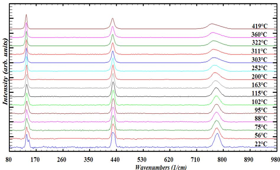
FIG. 4. Raman spectra of  $\text{Sr}_2\text{MgTeO}_6$  obtained for selected temperatures, as indicated.
