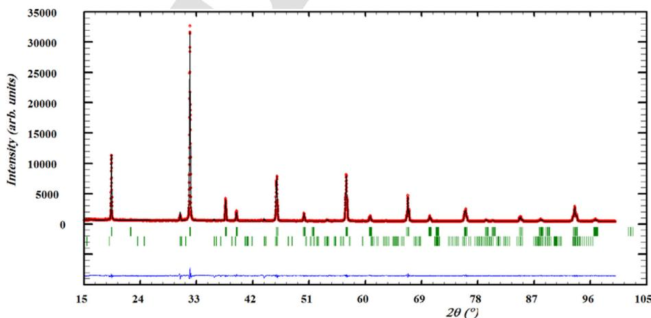
FIG. 1. Final Rietveld plots for monoclinic  $\text{Sr}_2\text{MgTeO}_6$ . The upper symbols illustrate the observed data (circles) and the calculated pattern (solid line). The vertical markers show calculated positions of Bragg reflections. The lower curve is the difference diagram. The non-indexed peaks are unidentified. The refined impurity is  $\text{MgTeO}_4$ .
