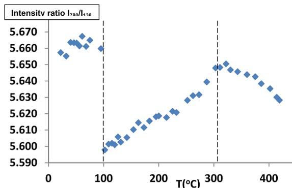
FIG. 6.  $I_{780}/I_{138}$  intensity ratio of two phonon modes in Raman spectra in  $\text{Sr}_2\text{MgTeO}_6$ . Two distinct changes occur at around 100 °C and 300 °C.
