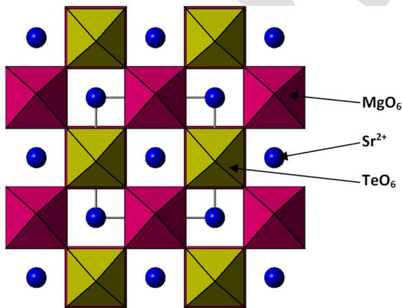
FIG. 2. A (001) projection of the unit cell indicates the typical polyhedral arrangement.
