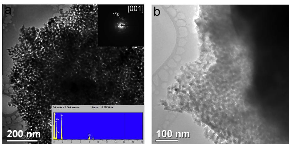
Fig. 3. (a, b) TEM image of mesostructured stishovite recovered from 14 GPa and 500 °C after plasma etching treatment with relative SAED and EDX spectrum (inset).
