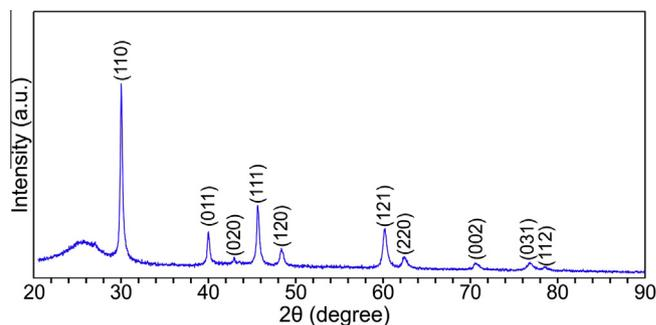
Fig. 1. X-ray diffraction pattern (Cu K $\alpha$  radiation) of recovered stishovite after 3 h at 14 GPa and 500 °C.
