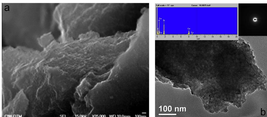
Fig. 2. (a) SEM and (b) TEM image of the recovered stishovite after 3 h at 14 GPa and 500 °C. SAED (inset) and EDX spectrum.
