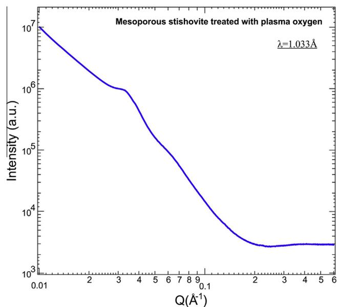
Fig. 4. SAXS pattern of stishovite recovered from 14 GPa and 500 °C after plasma etching treatment showing a weak periodicity.
