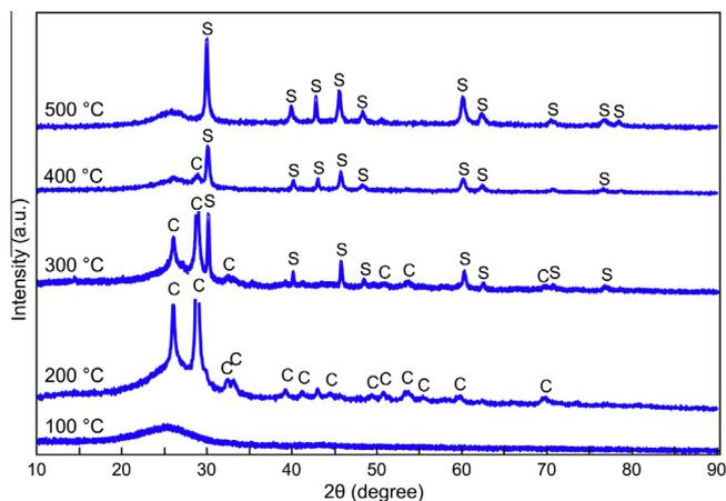
**Fig. 5.** XRD patterns (Cu  $K_{\alpha}$  radiation) relative to experiments performed at 14 GPa and temperatures of 100–500 °C showing the evolution of the crystalline nature of the recovered samples from FDU-12/C composite. The lowest temperature of crystallization for stishovite (s) is shown to be about 500 °C, while metastable coesite (c) is obtained directly from the amorphous precursor at about 200 °C. No peaks representative of crystalline form of carbon are observed.
