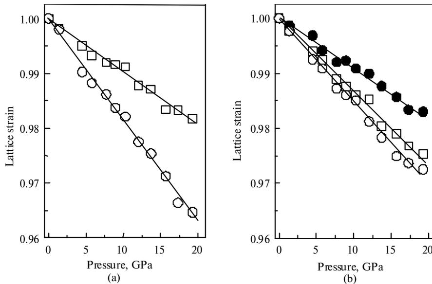
Fig. 5. Relative cell parameters as a function of pressure for (a)  $\text{CrB}_2$  and (b)  $\text{CrB}_4$  derived from high-pressure X-ray diffraction data. ( $\square$ )  $a/a_0$ , ( $\circ$ )  $c/c_0$ , ( $\bullet$ )  $b/b_0$ .
