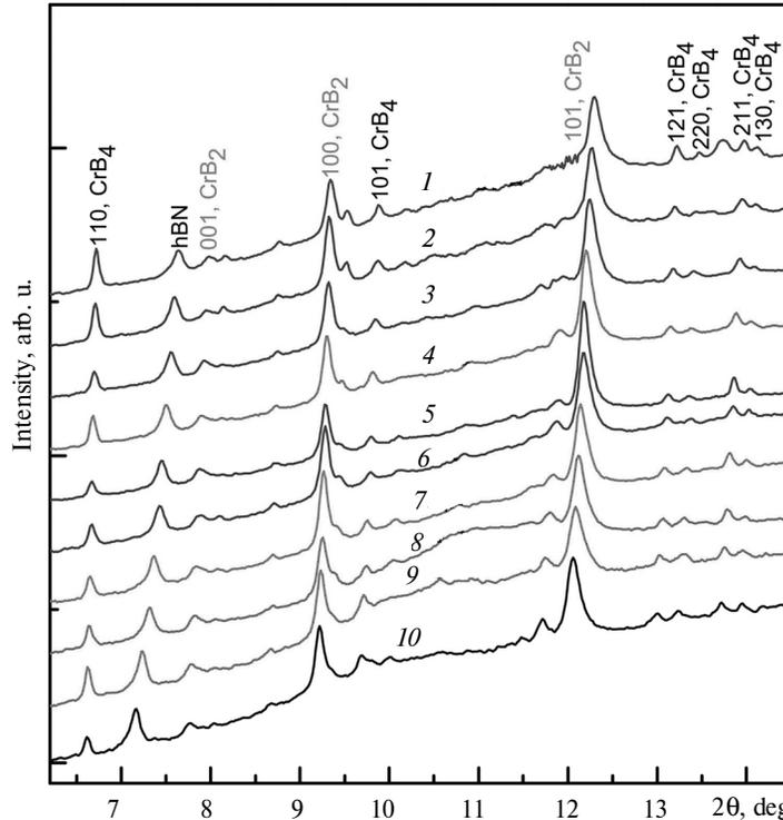
**Fig. 3.** Selected high-pressure synchrotron X-ray diffraction patterns collected at room temperature in a diamond-anvil cell: 15.7 (1), 13.6 (2), 12.0 (3), 10.2 (4), 8.9 (5), 7.7 (6), 5.8 (7), 4.5 (8), 2.8 (9), 1.4 (10) GPa. The incident X-ray wavelength is  $\lambda = 0.41326$  Å.
