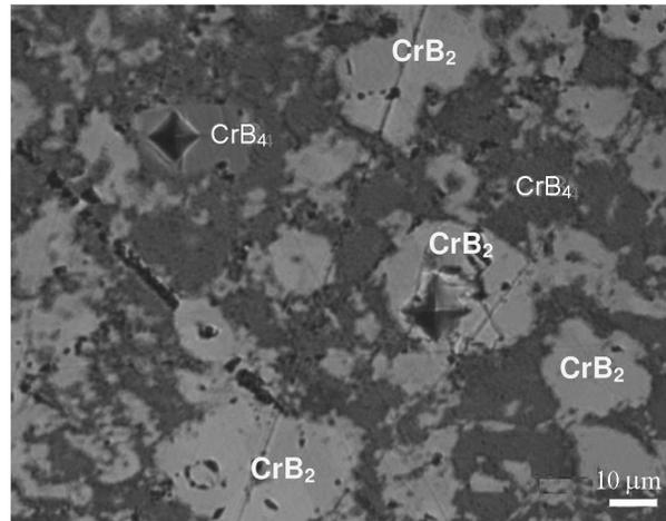
**Fig. 6.** A fluorescence image of the indentations produced at an indenter tip load of 200 g with a dwell time of 15 s. The dark and bright regions are  $\text{CrB}_4$  and  $\text{CrB}_2$ , respectively.
