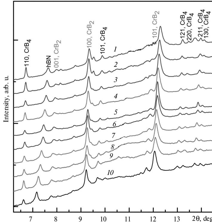
**Fig. 3.** Selected high-pressure synchrotron X-ray diffraction patterns collected at room temperature in a diamond-anvil cell: 15.7 (1), 13.6 (2), 12.0 (3), 10.2 (4), 8.9 (5), 7.7 (6), 5.8 (7), 4.5 (8), 2.8 (9), 1.4 (10) GPa. The incident X-ray wavelength is  $\lambda = 0.41326 \text{ \AA}$ .
