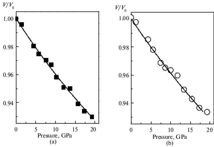
**Fig. 4.** Volume–pressure data fitted to the second order Birch–Murnaghan equation of state for (a)  $\text{CrB}_2$  and (b)  $\text{CrB}_4$ .
