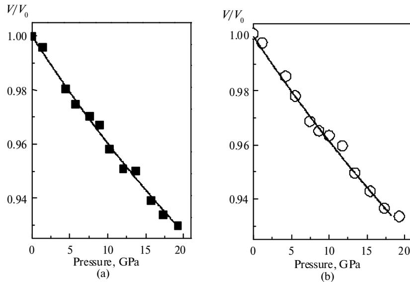
Fig. 4. Volume–pressure data fitted to the second order Birch–Murnaghan equation of state for (a)  $\text{CrB}_2$  and (b)  $\text{CrB}_4$ .
