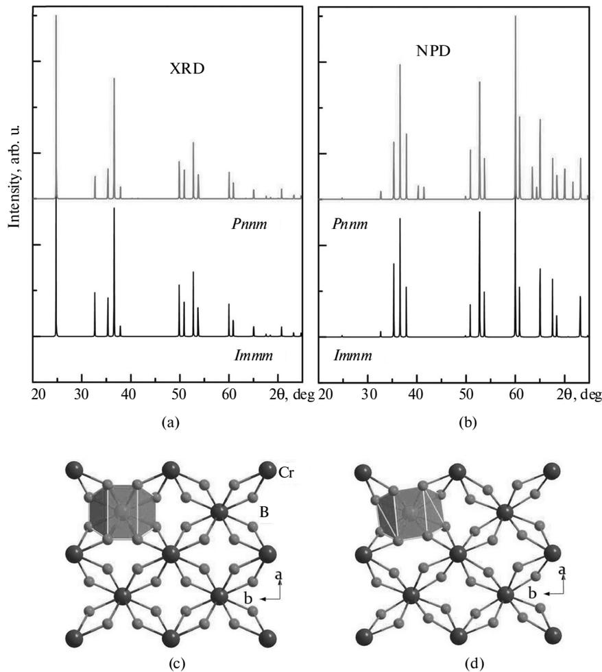
**Fig. 2.** (a) Simulated powder X-ray and (b) neutron diffraction patterns for CrB<sub>4</sub> based on two possible structures of *Immm* (no. 71) and *Pnmm* (no. 58). (c) Crystal structures of *Immm* and *Pnmm* (d) (see the table for structure details).
