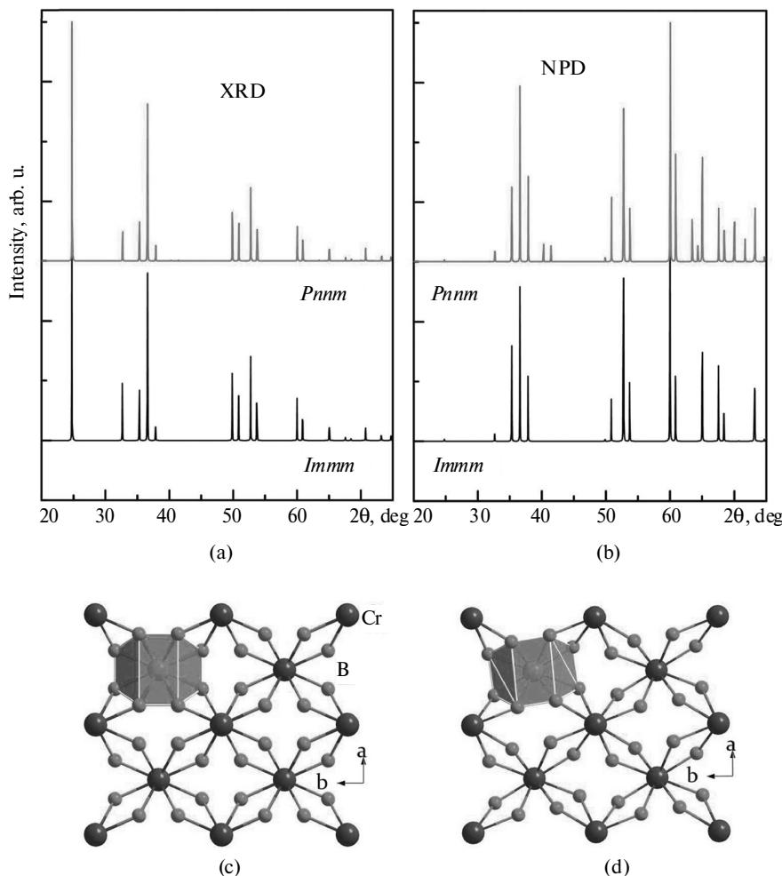
**Fig. 2.** (a) Simulated powder X-ray and (b) neutron diffraction patterns for CrB<sub>4</sub> based on two possible structures of *Immm* (no. 71) and *Pnnm* (no. 58). (c) Crystal structures of *Immm* and *Pnnm* (d) (see the table for structure details).
