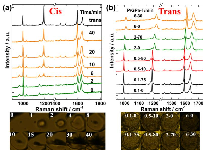
**Figure 5.** Selected *in situ* Raman patterns of (a) cis → trans-stilbene at 0.5 GPa by 532 nm laser irradiation, and (b) trans → cis-stilbene by 360 nm laser irradiation at different pressures; the pictures at the bottom correspond to the spectra at the top.
