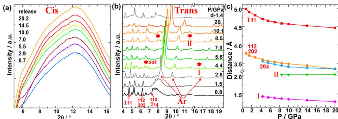
**Figure 4.** Selected *in situ* XRD patterns of cis-stilbene (a) and trans-stilbene (b) under high pressure. (c) The main XRD peaks of trans-stilbene vary with pressure.
