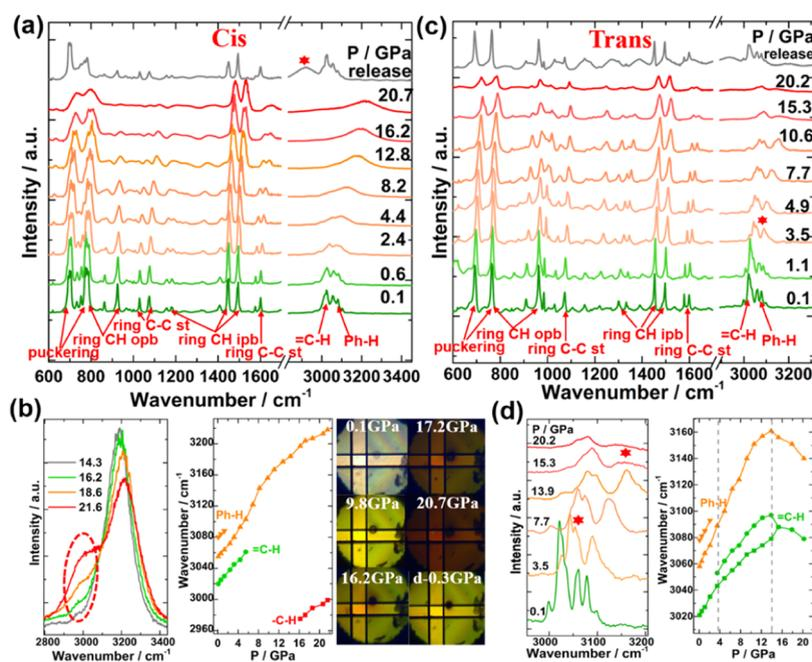
**Figure 1.** (a) Selected IR spectra of cis-stilbene under high pressure, (b) C–H stretching peak of cis-stilbene changes with pressure higher than 12.8 GPa (left panel), the peak position of the =C–H stretching vibration changes at 0–20.7 GPa (middle), and there is a color change in the sample (right panel). (c) Selected IR spectra of trans-stilbene. (d) Details of the =C–H stretching peak and the peak position of trans-stilbene as a function of pressure.
