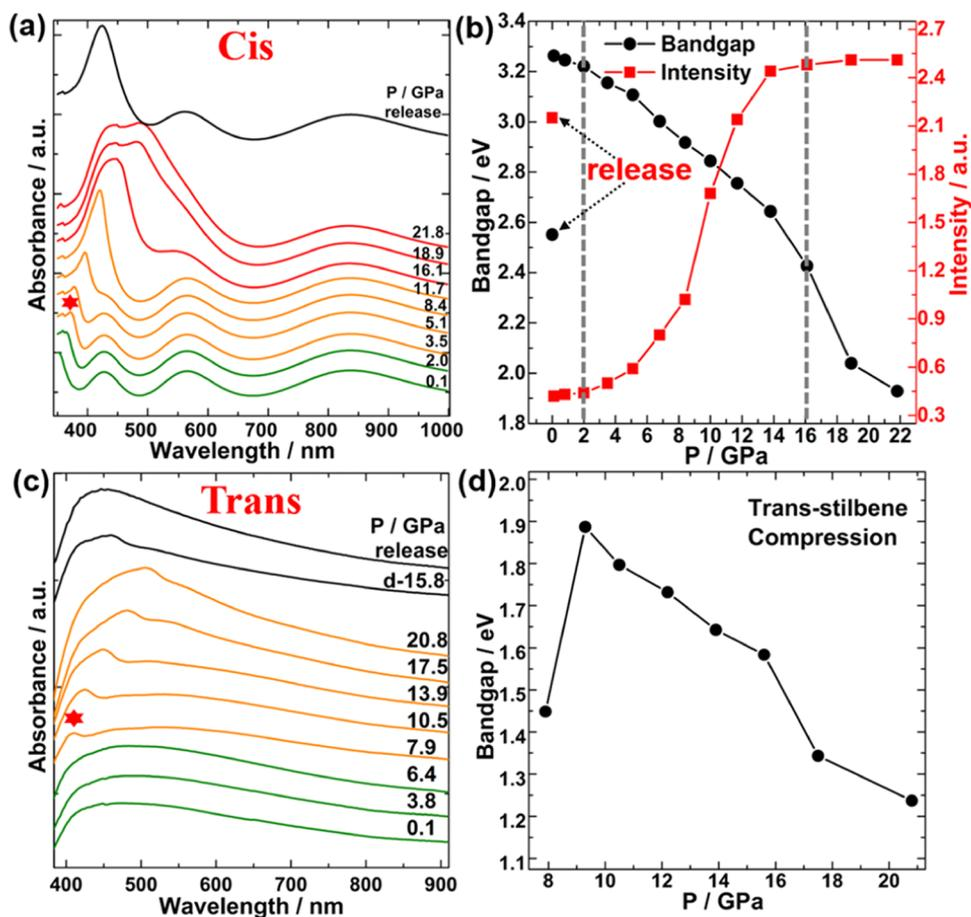
Figure 3. (a) Selected *in situ* UV-vis patterns of cis-stilbene under high pressure. (b) Variation of band gap and peak intensity of cis-stilbene with pressure, and these two isolated points at ambient pressure represent the band-gap value and the intensity value released to ambient pressure. (c) Selected *in situ* UV-vis patterns of trans-stilbene under high pressure. (d) Band gap of trans-stilbene under high pressure.
