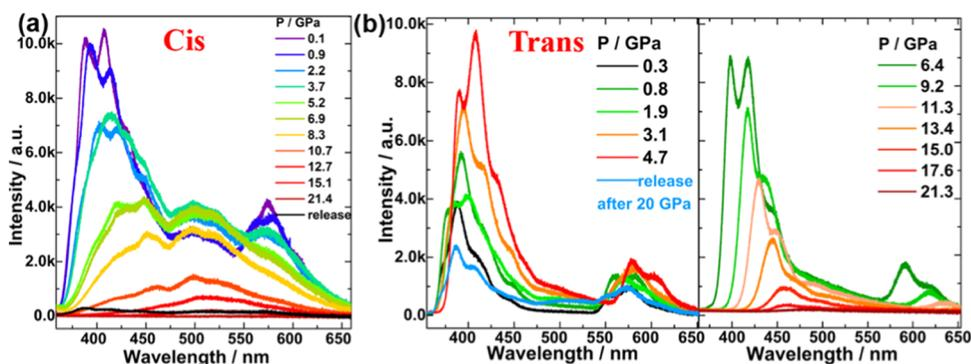
Figure 2. Selected fluorescence spectra of (a) cis-stilbene and (b) trans-stilbene under different pressures.
