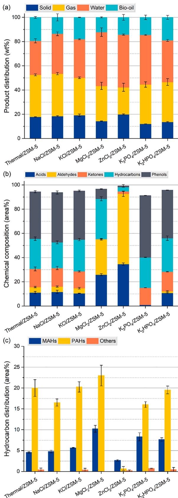
Fig. 2. Effect of inorganic salts on the (a) product distribution, (b) bio-oil composition, and (c) hydrocarbon production.
