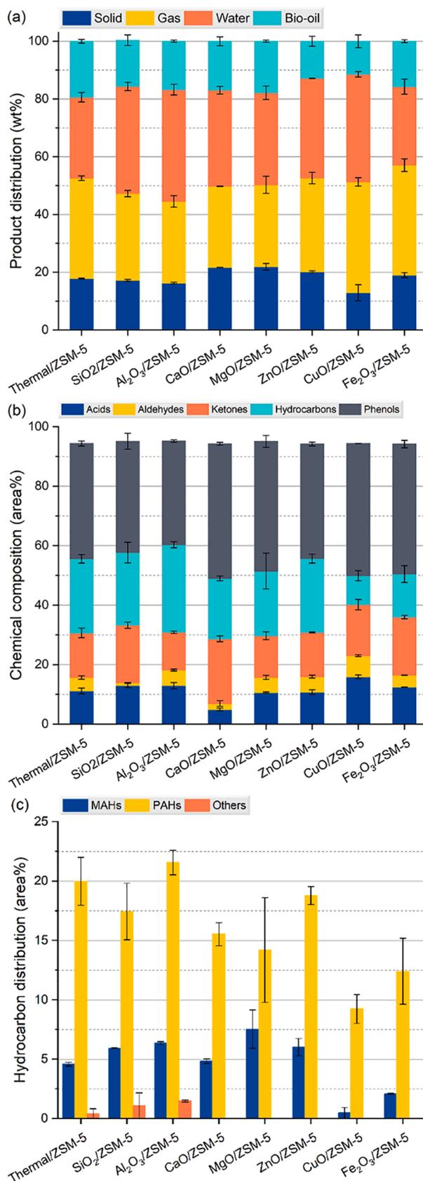
Fig. 3. Effect of metal oxides on the (a) product distribution, (b) bio-oil composition, and (c) hydrocarbon production.
