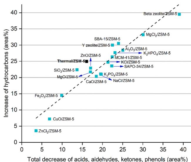
Fig. 7. The selectivity reduction of oxygenates as a function of the selectivity increase of hydrocarbons over all the catalyst combinations.
