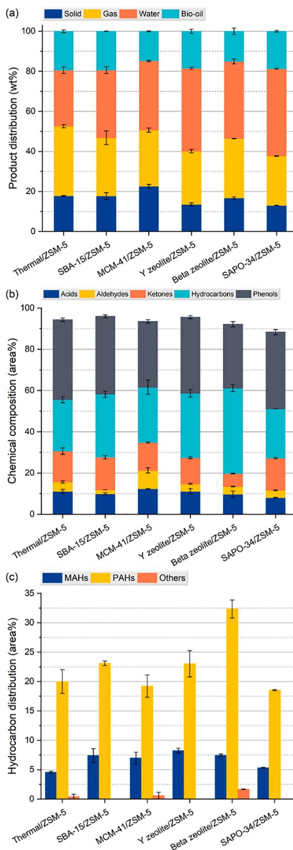
Fig. 4. Effect of porous materials on the (a) product distribution, (b) bio-oil composition, and (c) hydrocarbon production.
