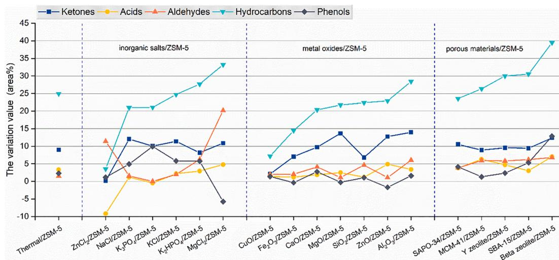
Fig. 6. Chemical selectivity variation impacted by the secondary ZSM-5 catalyst for all the first-layered catalysts. Note: the ordinate represents the increase of hydrocarbons and reduction of ketones, acids, aldehydes, and phenols.
