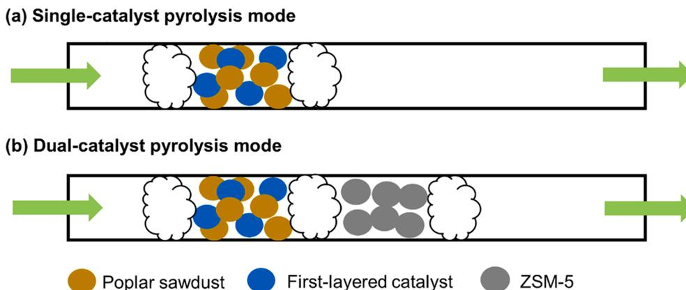
Fig. 1. Schematic diagram of the single-catalyst and dual-catalyst CFP modes.
