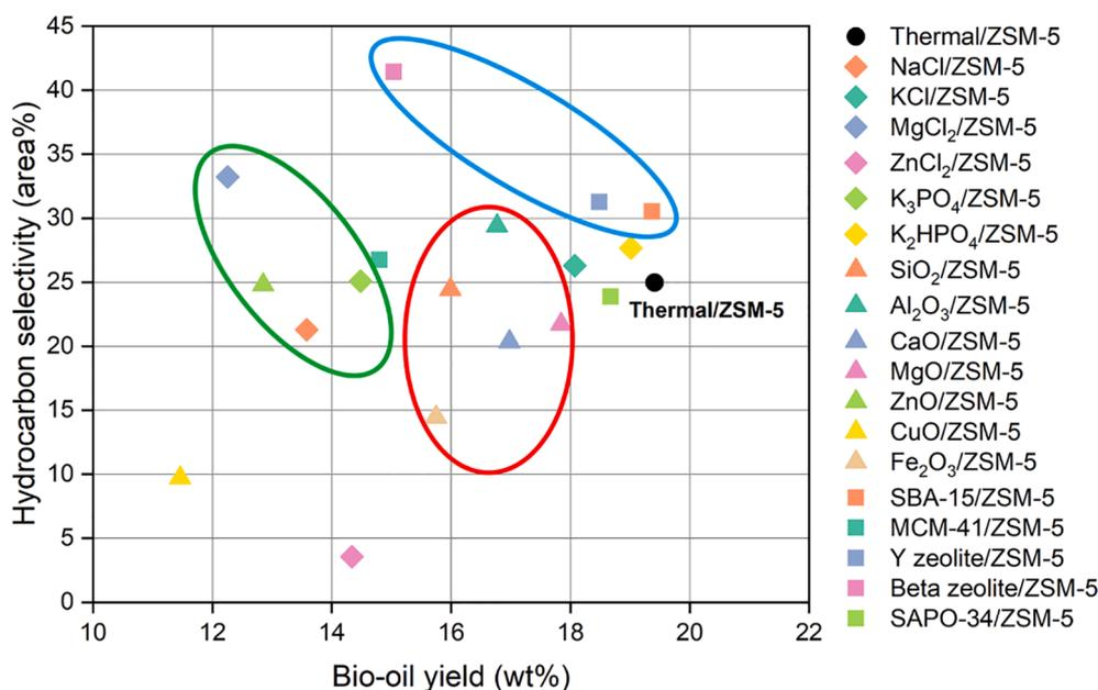
Fig. 5. The comparative catalytic activity of all the first-layered catalysts in combination with ZSM-5. The inorganic salts, metal oxides, and porous materials are circled in green, red, and blue, respectively.
