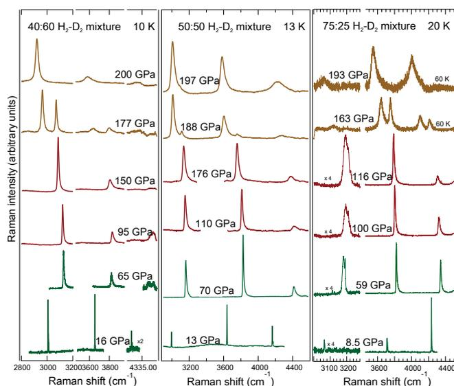
**Fig. 4.** Representative vibrational Raman spectra of (Left) 40:60, (Middle) 50:50, and (Right) 75:25 H<sub>2</sub>-D<sub>2</sub> mixtures as a function of pressure at 10, 13, and 20 K, respectively. Colors indicate phase I (green), phase II (red), and phase III (orange).
