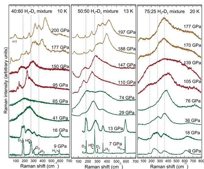
**Fig. 3.** Representative low-frequency Raman spectra of (Left) 40:60, (Middle) 50:50, and (Right) 75:25 H<sub>2</sub>-D<sub>2</sub> mixtures as a function of pressure at 10, 13, and 20 K respectively. Colors indicate phase I (green), phase II (red), and phase III (orange).
