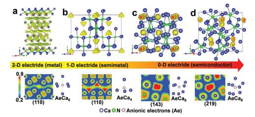
Figure 5. Calculated electron localization functions (ELFs) for a)  $R\bar{3}m$ , b)  $Fd\bar{3}m$ , c)  $I\bar{4}2d$ , and d) Cc structures with isosurface value 0.55, 0.9, 0.9, and 0.9, respectively. The ELF maps around anionic electrons accompanied with the coordination environment of anionic electrons (Ae) are showed in the bottom. The distribution of anionic electrons reveals a transition from 2D layer  $(R\bar{3}m)$ , 1D chain  $(Fd\bar{3}m)$ , and 0D spheres  $(I\bar{4}2d$  and Cc).
