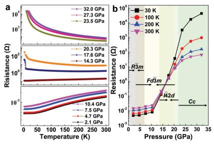
**Figure 3.** Electrical resistance changes with pressure and temperature. a) Temperature dependence of electrical resistance from 2 to 300 K. The curves obtained under pressures show the temperature dependence of electrical resistance changed from positive to negative. b) Electrical resistance values as a function of applied pressure at different temperature of 30, 100, 200, and 300 K, respectively.
