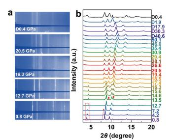
**Figure 1.** Synchrotron XRD patterns of  $Ca_2N$  obtained under compression up to 50.1 GPa and decompression. a) The raw 2D XRD images at selected pressures during compression and decompression. b) Integrated XRD profiles under different pressures.
