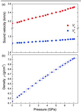
FIG. 2 (color online). Density measurement of L62 BMG using integrated ultrasonic sound velocity, x-ray radiography, and XRD measurements. (a) The sound velocities of the compression wave  $(V_p)$  and shear wave  $(V_s)$  as a function of pressure up to 7.1 GPa. (b) The density as a function of pressure obtained by calculation from ultrasonic sound velocities. The dotted line represents the fitting of density data using the third-order BM-EOS.
